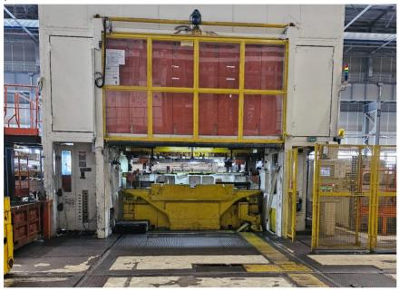
During the blanking of the A5U sidepanel on this blanking line several scraps are cut from the blank and fall into scrap chutes in the front and rear of the moving bolster. The picture below shows a top view of the blanking die. To increase the material utilization rate the front door scrap (circeled in green; now referred to as *the scrap*) has to be recovered for further processing.
