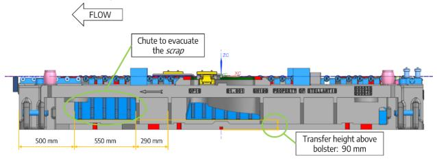
The scrap recovery device must take over *the scrap* at this handover point, convey it through the lifting gate and stack it on a blank pallet outside the press.
