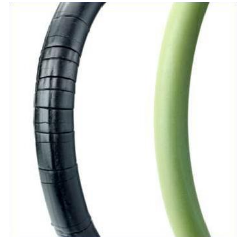
O-rings in nitrile (left) and Viton (right) after test at 200 °C
