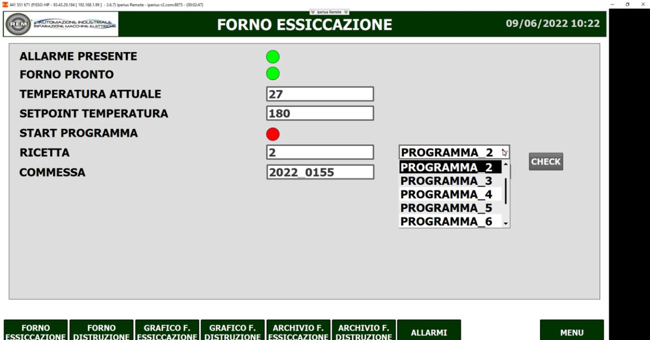
The screenshot shows a control interface for a 'FORNO ESSICCAZIONE' (Drying Oven). The interface includes a status bar at the top with the date and time '09/06/2022 10:22'. Below this, there are several parameters and their values:
