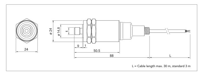
The 4-20 mA vibration transmitters are accelerometers that provide a 4-20 mA output signal proportional to the true RMS value of vibration velocity. The transmitters can be connected to common process control systems (PLC, DCS). The electrical signal is isolated from the transmitter housing. The transmitters operates by using power from a standard 4-20 mA loop.
