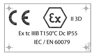
Figure 3-2 Ex plate on the machine (schematic representation)
