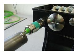
Figure 6-6 Slide the protective tube to remove the signal connector over the signal connector
