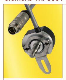
Designed as a drop in replacement for the Siemens 1XP8001 encoder, the EXC is ready for delivery. The unique threaded shaft made this encoder hard to nd, but now it is a standard order. Con gurations can be with either 1024 or 2048 CPR, with a 12 pin connector with 18" of extra cable. Save time and money looking for a replacement encoder; The EXC-8001/1024 is the perfect solution!
