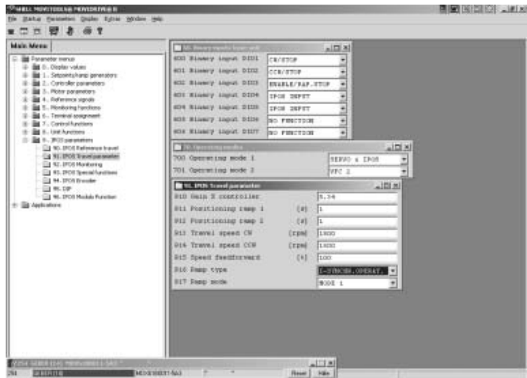
Figure 37: Parameter settings in the Shell program for starting up internal synchronous operation
