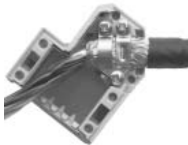
Figure 8: Connect the shield in the sub D connector
