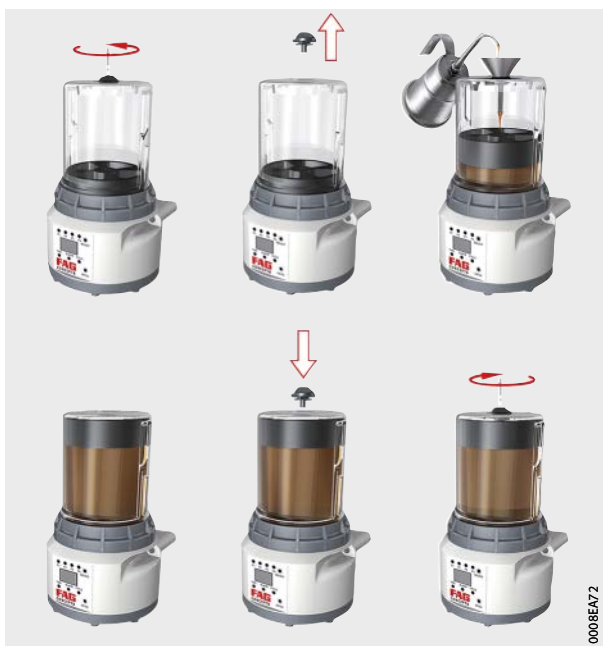
Figure 60 Refilling the oil reservoir
