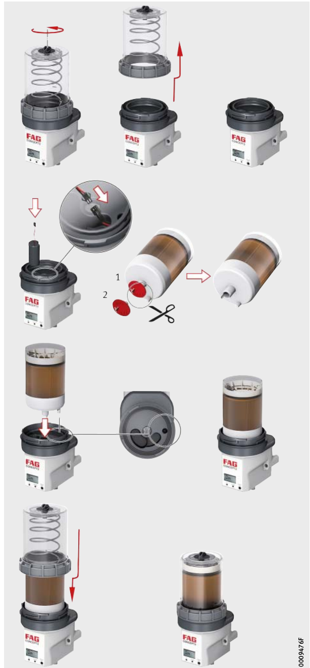
Figure 10 Connecting the battery and fitting the lubricant cartridge
