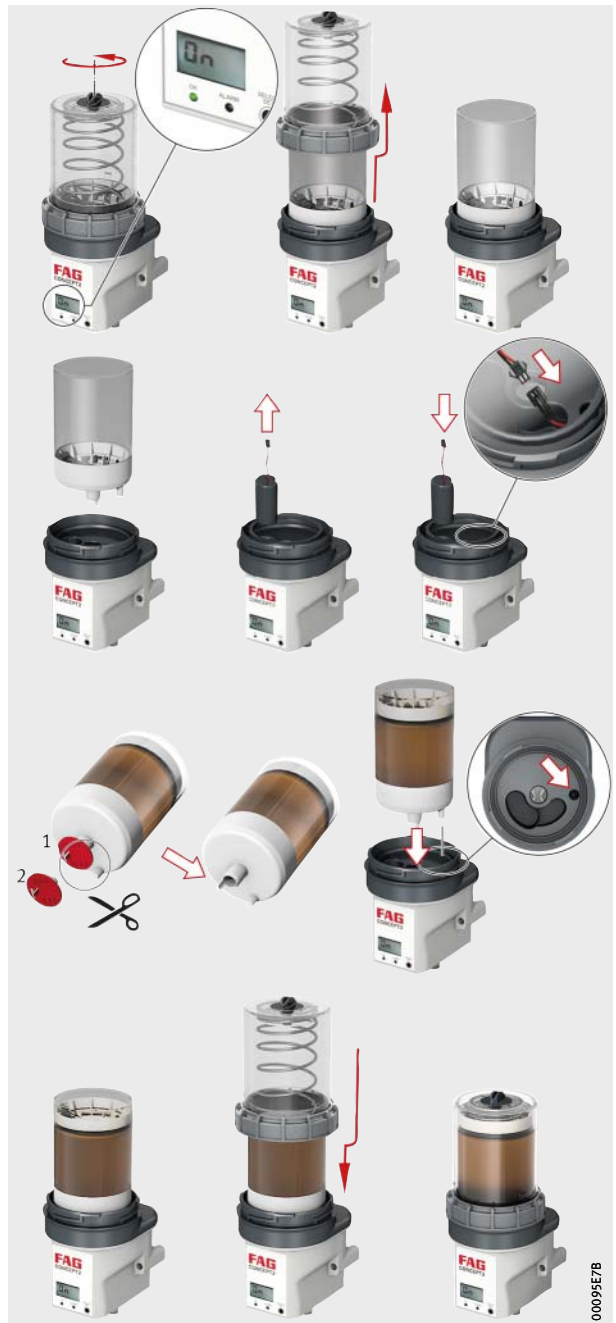
Figure 20 Replacing the cartridge and battery
