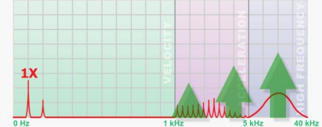
Stage Two: High Frequency Envelope, Demodulation and Acceleration Spectrum
