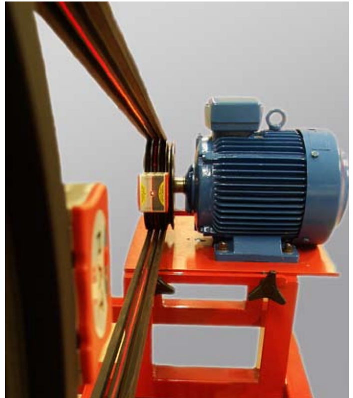
The visible red laser line makes it easy to determine the positions of your belt driven machines.
