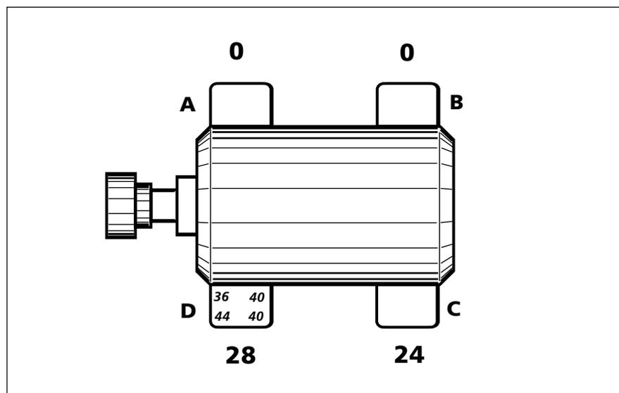
Two large OPTALIGN PLUS readings on one side with opposite side near zero cause suspicions of induced soft foot. Feeler gauge readings are taken at foot D (with the largest OPTALIGN PLUS value). Presence of parallel gap at foot D supports these suspicions. Presence of parallel gap at foot C as well would prove induced soft foot.
