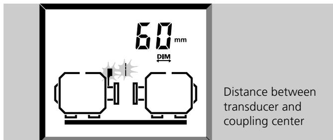
Measure from the marking on the top of the transducer housing to the coupling center. (For spacer couplings, enter additionally the spacer shaft length when both coupling symbols flash - see page 4-30.)
