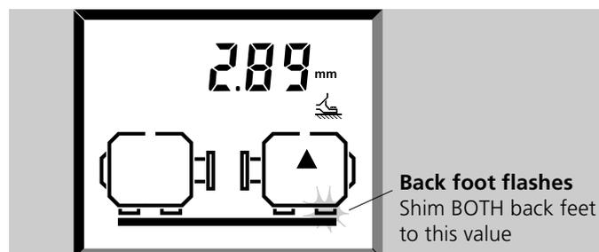
Shim BOTH back feet to the on-screen value, trying not to move the machine horizontally.
