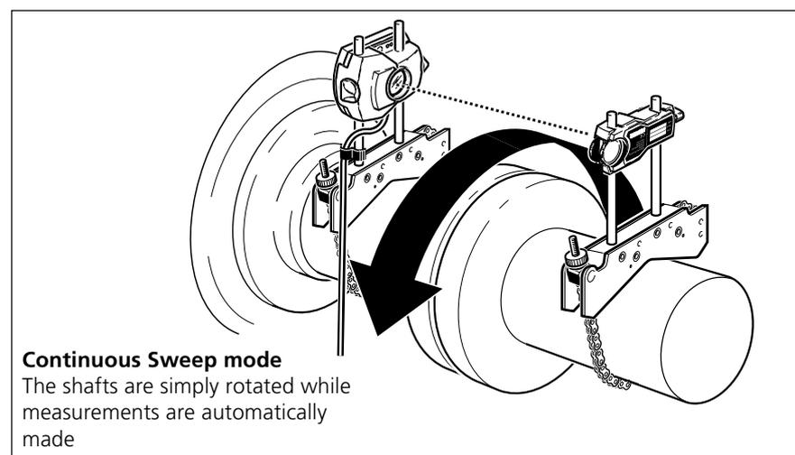
This is the measurement mode described in the standard horizontal alignment procedure (page 3-22) and is recommended for most standard cases.
