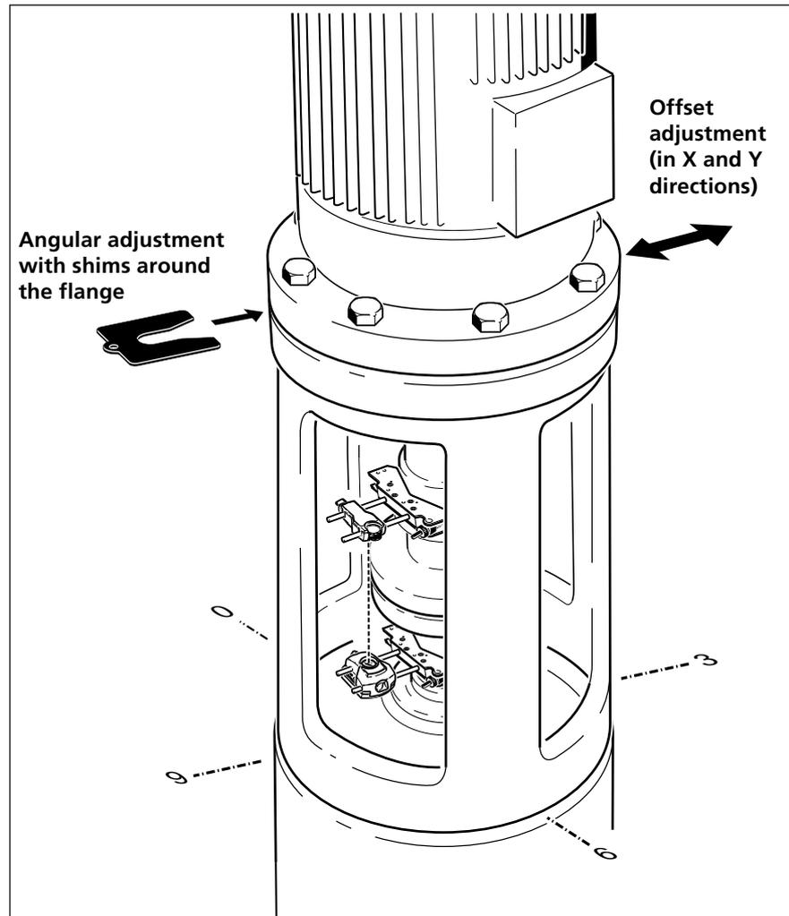
The OPTALIGN PLUS transducer and reflector are mounted on either side of the coupling as for horizontal machines, with the transducer below and the reflector above. Measurements are then made at a series of  $90^\circ$  or  $45^\circ$  rotational positions.
