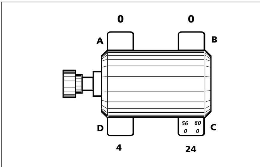
Feeler gauge readings are taken to examine the foot with the high OPTALIGN PLUS reading, and a bent foot is found. It is possible that other feet have problems that are being masked by foot C.
