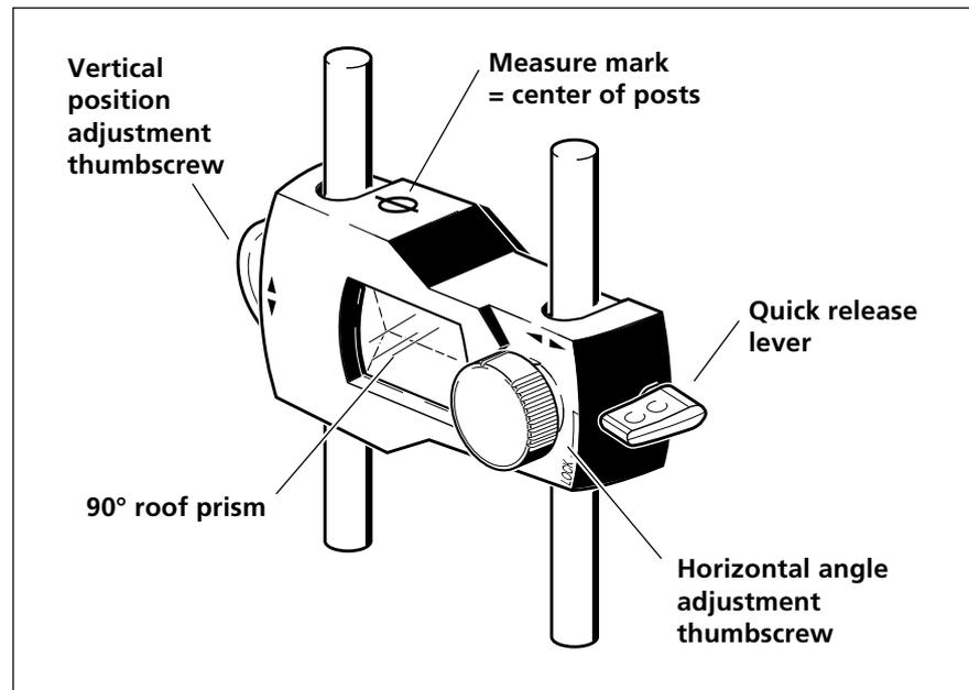
The reflector must be kept clean. Use the ALI 2.905 cleaning set or a fine dusting brush such as that normally used to clean other optical devices.
