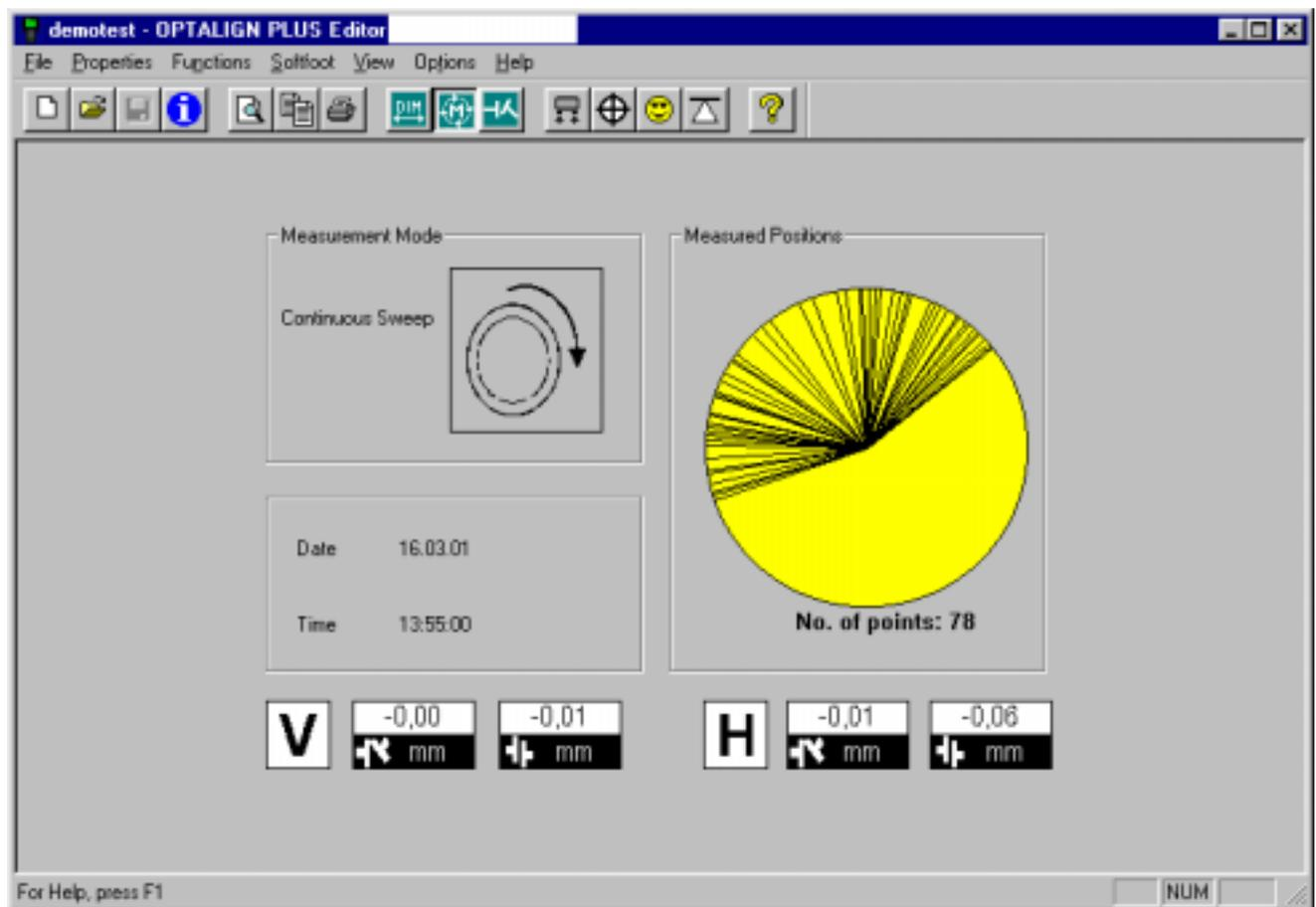
The bottom portion shows the calculated alignment condition at the coupling.
