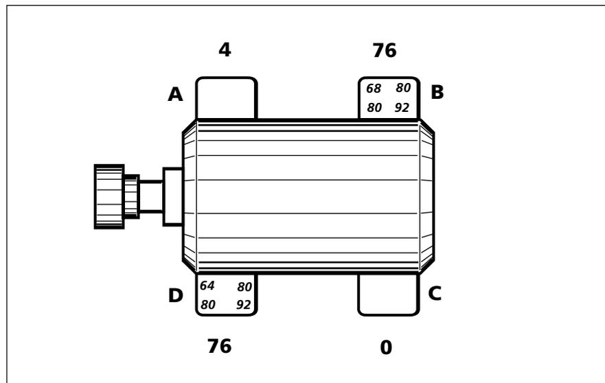
Identical OPTALIGN PLUS readings to example 2. Feeler gauge are used to examine feet B and D. Feeler gauges indicate equal rock, but definite slope from foot C to foot A. This suggests that foot C is out of plane compared to feet A, B and D.
