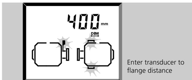
Enter the distance between the marking on the top of the transducer and the center surface of the flange.
