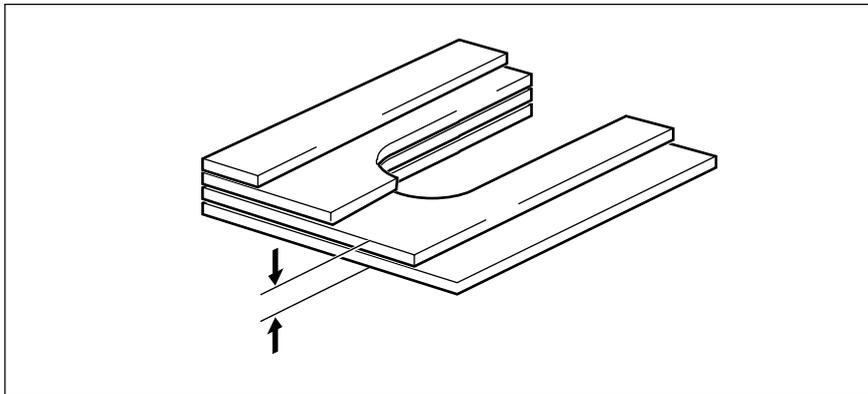
If the soft foot is purely 'angular' then the stepped shim will vary in thickness from about zero to twice the displayed OPTALIGN PLUS value.
