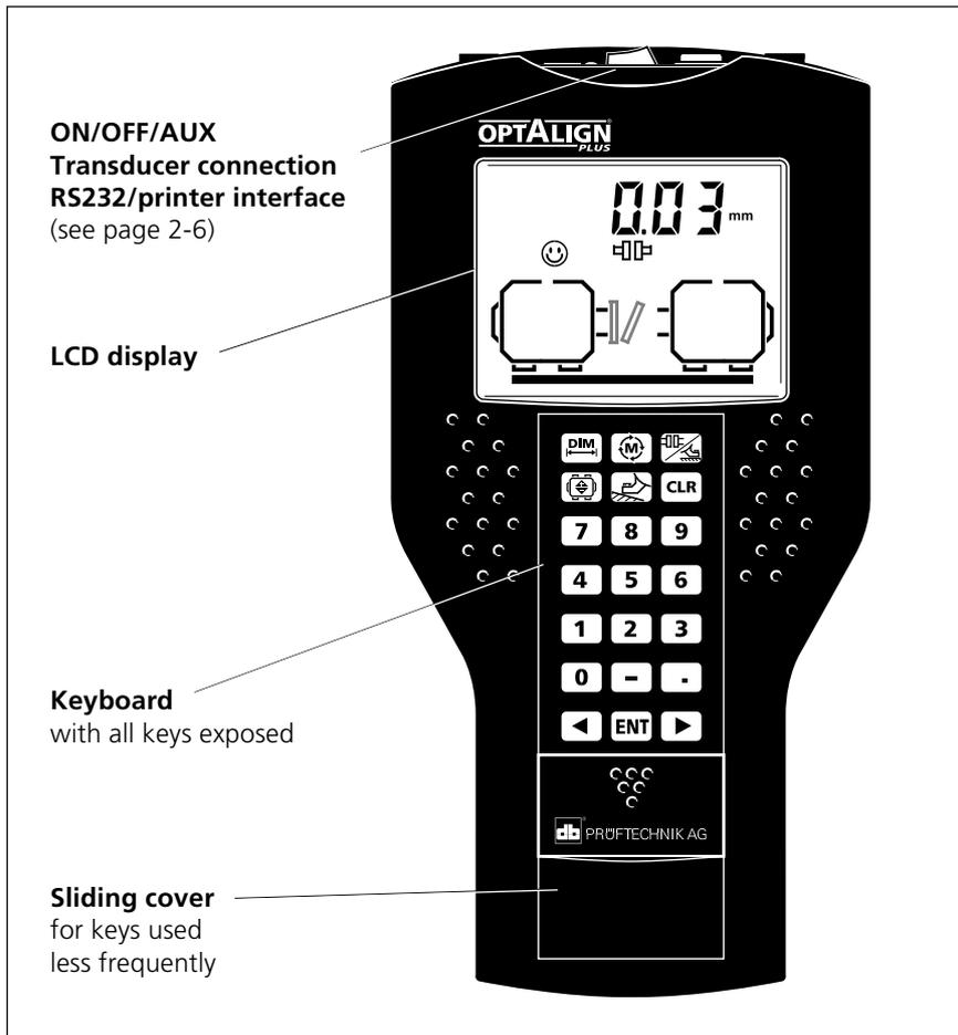
The heart of the OPTALIGN PLUS system is the OPTALIGN PLUS Control Unit, built to rugged industrial standards of shock and water resistance (IP65). It features an easy-to-read, energy-saving fixed-segment LCD display and numeric-function keypad.
