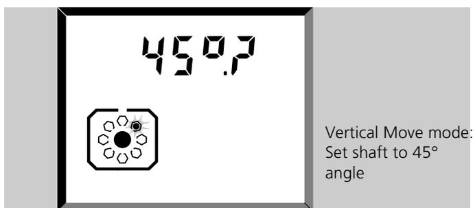
The screen shows **45°?** Rotate the shaft to the 45° position (1.30 o'clock). Note that the internal inclinometer is not operational during alignment of vertical machines, so positioning must be done manually.
