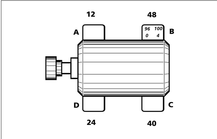
One foot having high OPTALIGN PLUS readings prompts feeler gauge examination of foot B. The feeler gauge readings show a clearly defined bent foot. It is possible that all of the other readings are being induced by the bend in foot B.
