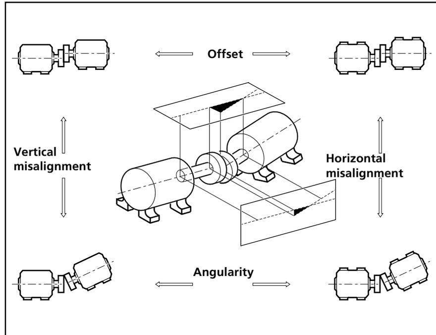
Any misalignment between the two machine shafts, as shown above, may be considered in terms of four basic alignment parameters:
