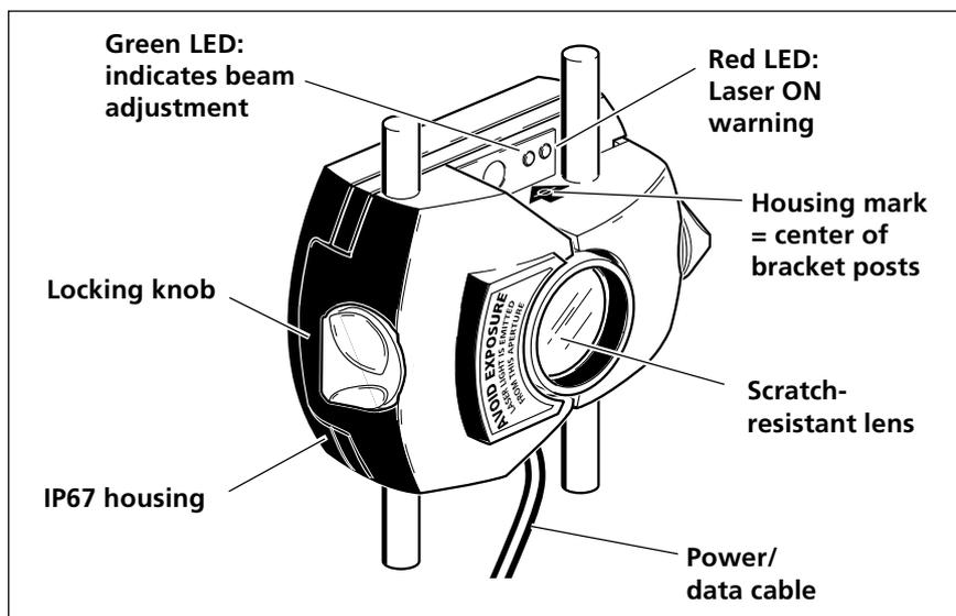
As with all the OPTALIGN PLUS components, the transducer is IP67 protected to resist water spray and dust. The internal optics and electronics are sealed to prevent any possible contamination. The transducer lens, however, must be kept clean. Use the ALI 2.905 cleaning set or a fine dusting brush such as that normally used to clean other optical devices. Keep the dust cap on when not in use.
