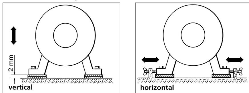
If the machine to be moved stands directly on the foundations, it cannot be lowered for alignment correction. Therefore, it is generally advisable to start with about 2 mm (80 mils) of shims beneath the feet of both machines.
