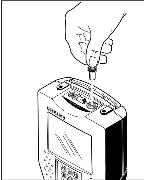
Insert the straight-ended cable plug into the eight-pin socket on the top of the control unit housing, with the arrow at the front.
