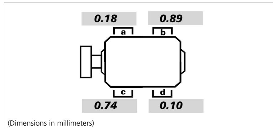
In the above example the correction would be to place a 0.89mm shim under foot 'b' (the foot with the largest gap) - just like placing a matchbook under the short leg of a wobbly table!
