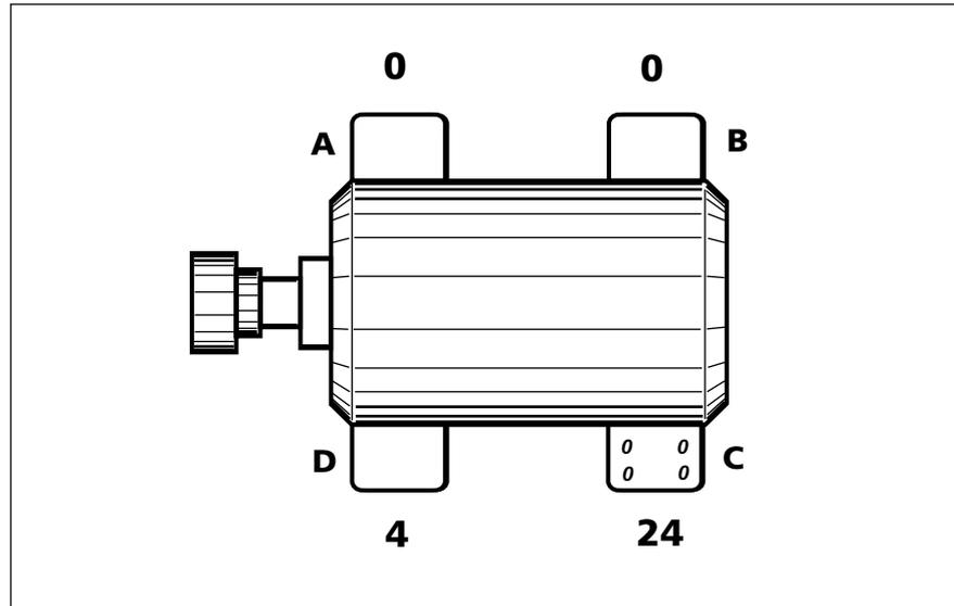
Feeler gauges are used to examine the foot with the largest OPTALIGN PLUS reading, but no gap is found.
