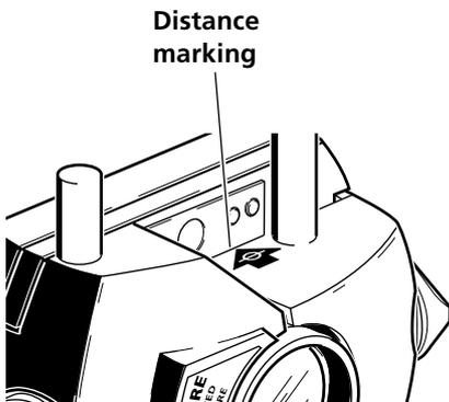
The screen prompts for the distance between the markings on the tops of the transducer and reflector:
