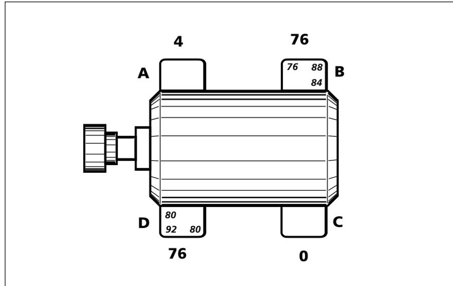
Identical and opposing OPTALIGN PLUS readings prompt feeler gauge examination of feet B and D. Feeler gauges indicate equal rock from one foot to another. Feet B and D are equally out of plane with feet A and C. The inside feeler gauge readings were left out of this example because they are often impossible to take in the field.
