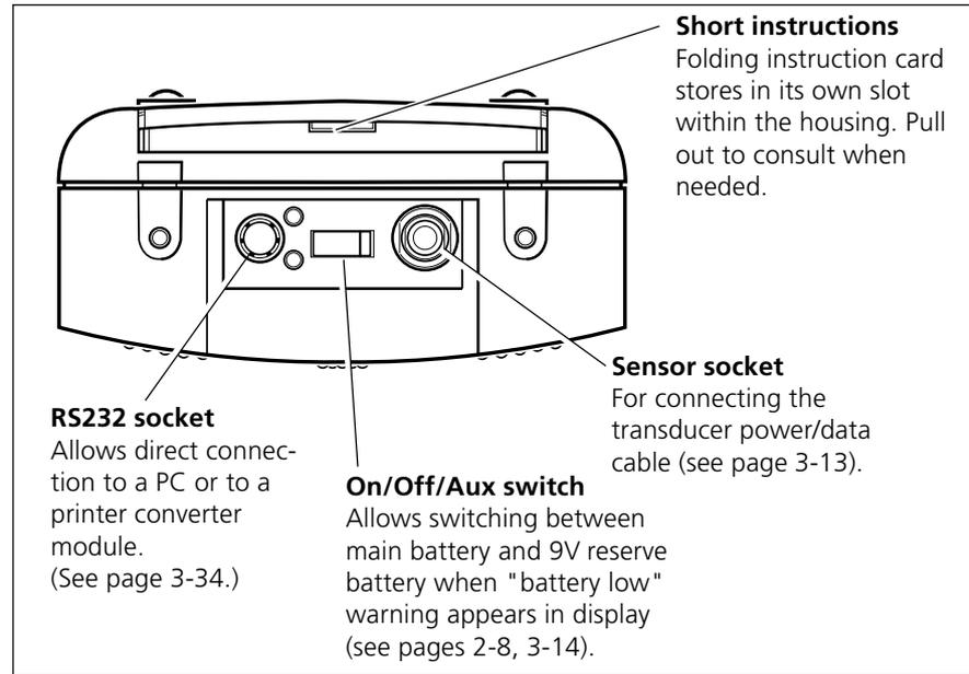
**Transducer connection & RS232/printer interface**
