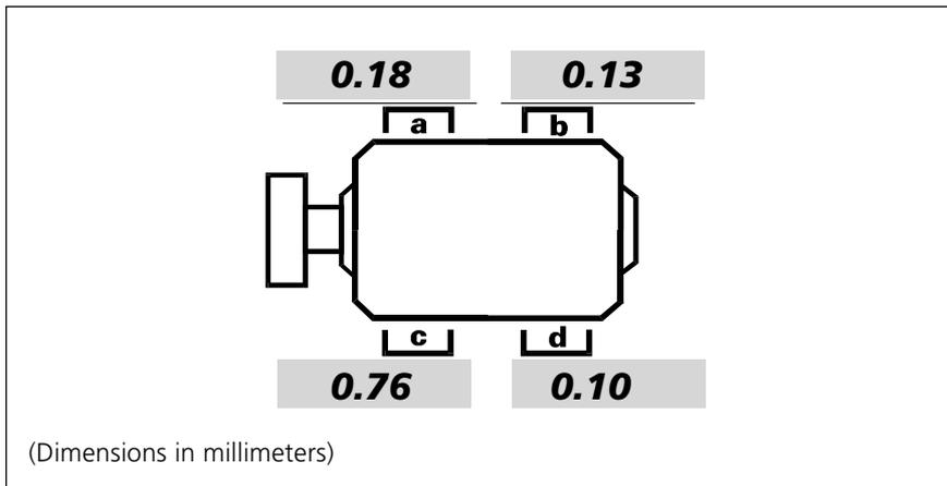
The 'problem foot' or machine frame is probably bent or distorted in some way. In this case loosen the bolt and examine the foot more closely. Use a feeler gauge to establish the variation of the gap and use these measurements to sketch the shape and dimensions for a stepped shim:
