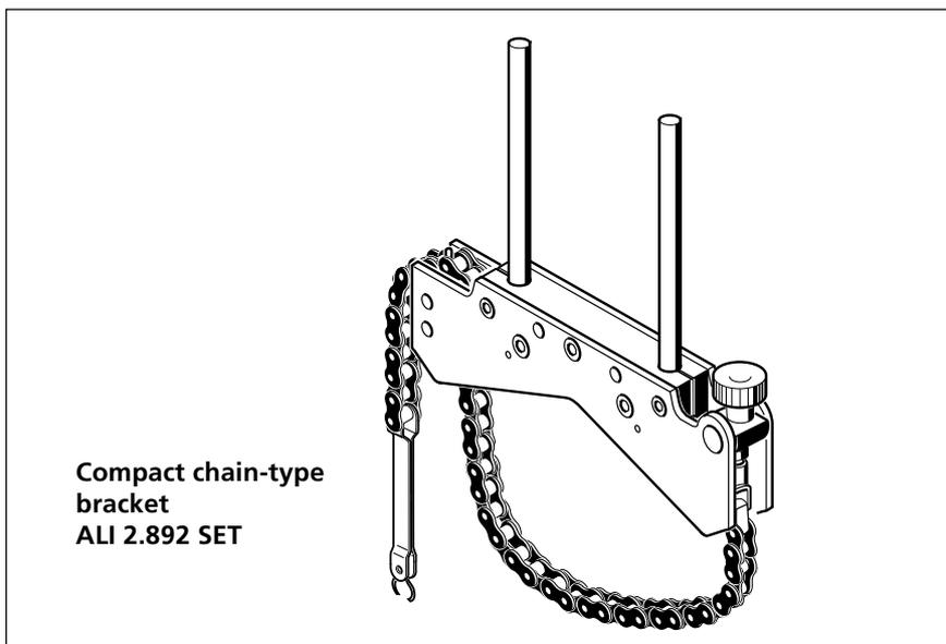
Compact and lightweight, this bracket is designed to provide extremely rigid support for the measurement components with a minimum of mounting time and effort. The compact chain-type bracket fits onto shafts and couplings ranging from 15 to 500 mm (1/2" to 20") in diameter. Longer chains are also available. Mounting instructions are given on page 3-8. Other bracket types are also available; these are described in chapter 6.
