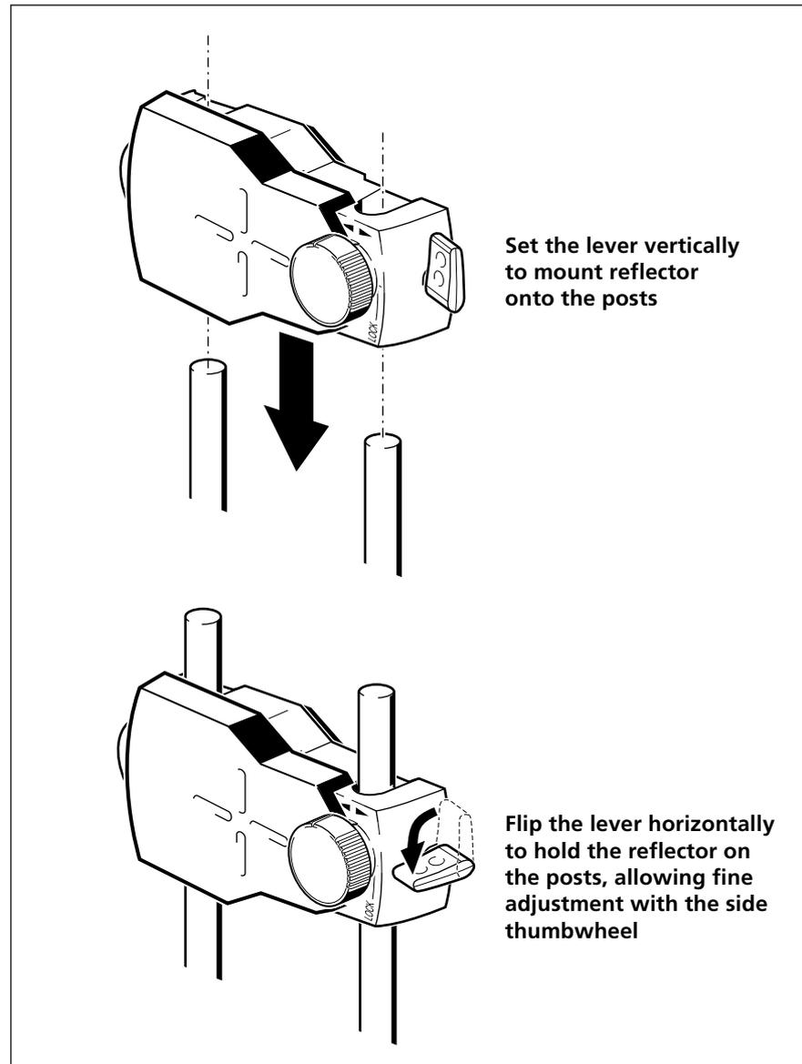
Both transducer and reflector should be at the same height, as low as possible, yet just high enough for the beam to clear the coupling flange. They should also appear parallel to each other by eye.
