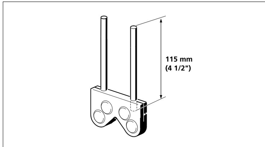
Wipe any traces of grease or oil from the mounting surface to avoid bracket slippage (which would reduce measurement accuracy).
