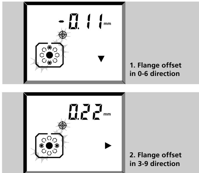
The arrow indicates the direction of the required correction. Use the OPTALIGN PLUS Move function to make these adjustments, page 5-16.
