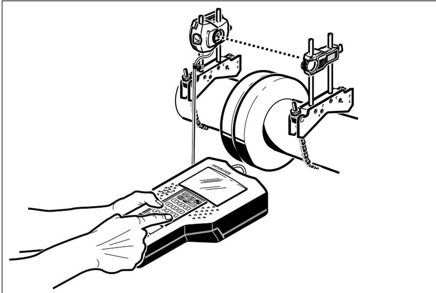
To measure the misalignment, the shafts are rotated. The laser beam is reflected by the reflector back into the transducer, where it strikes the position detector. During rotation, any shaft misalignment causes the laser beam to change its position in the detector.
