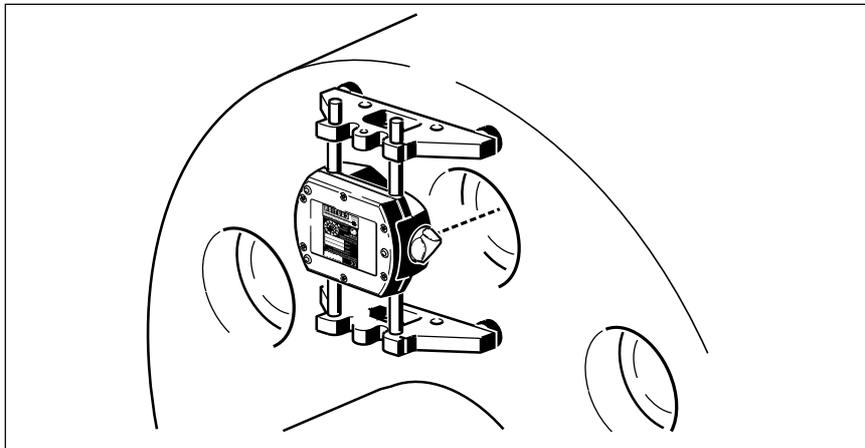
Use only the 115 mm (4½") support rods supplied with the bracket. The position of the support rods may be changed by loosening the hex screws which clamp them in the bracket.
