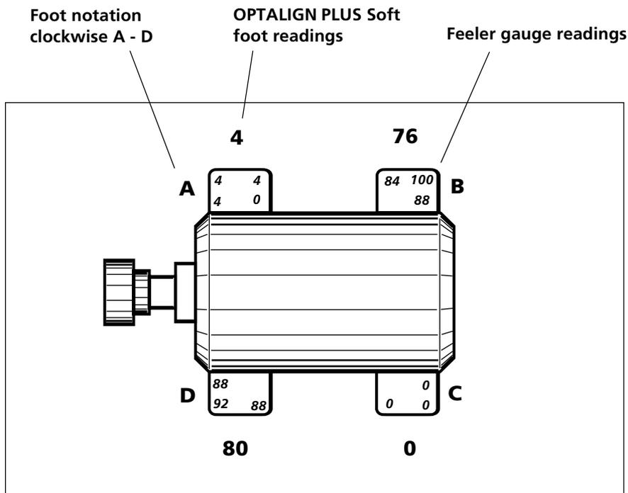
OPTALIGN PLUS readings show near perfect rock, tempting the inexperienced aligner to shim feet B and D. In this case, that would be a mistake. The 4/100 mm difference diagonally, with near zero readings on the other diagonal, prompts feeler gauge examination of feet B and D. The feeler gauge results show very similar average gaps between feet B and D but one is plainly sloped while the other is nearly flat.
