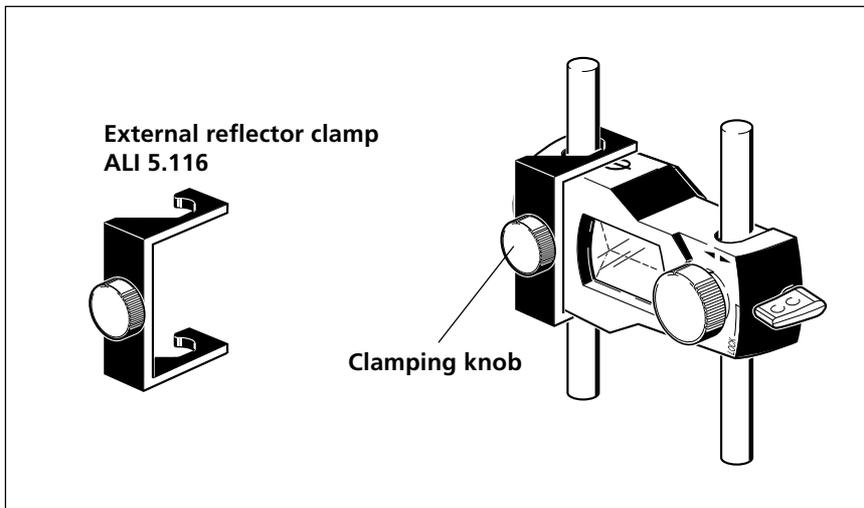
Once the reflector is adjusted, attach the clamp as shown above, then tighten down the clamping knob to lock the reflector in place.
