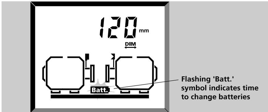
Save your current data if required (page 3-34) and switch off the control unit before changing batteries. Open the back panel to see the batteries, thus:
