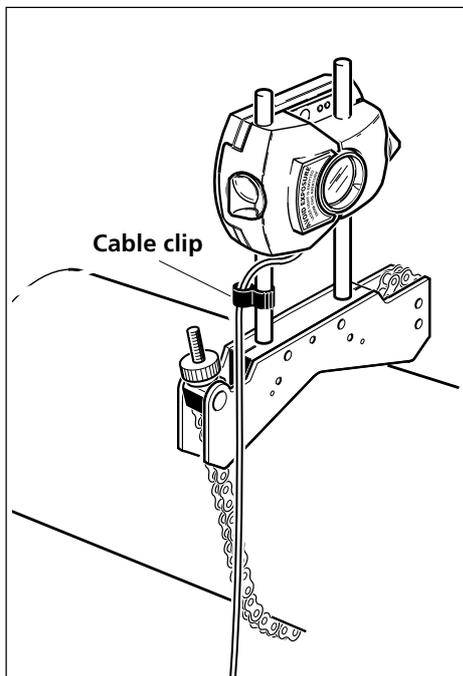
The cable is permanently attached to the transducer. In case of damage, it may be replaced as directed in the appendix (chapter 6).
