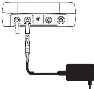
Connect the VIBXPERT charger either to channel A or to channel B.
