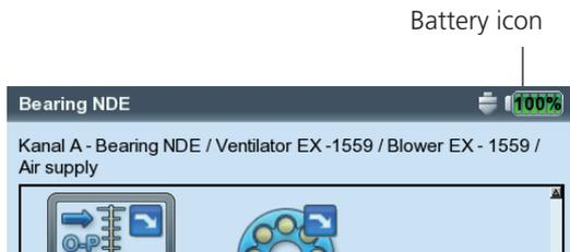
If the battery is almost empty, a message appears on the display and the blue LED flashes. The battery can be charged either in the device or in the external charging station (option, VIB 5.324) using the VIBXPERT charger (VIB 5.320-INT).
