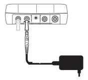
Connect the VIBXPERT charger either to channel A or to channel B.
