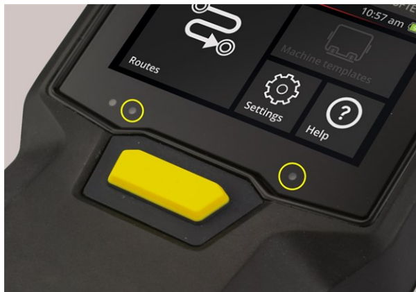
Two inlet openings for ambient light sensor.
