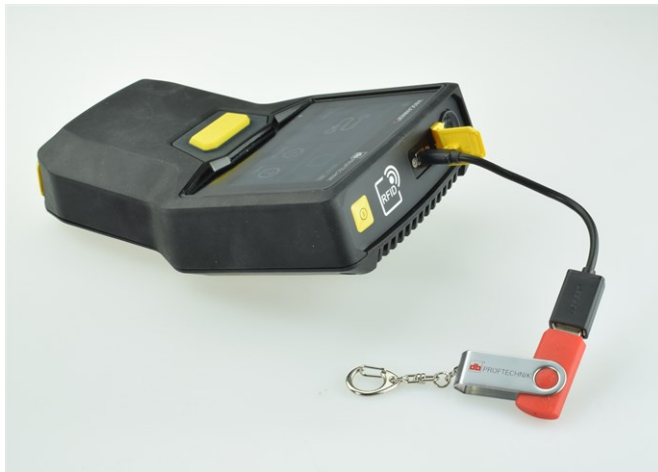
USB pendrive with adapter connected to the VIBSCANNER 2.
