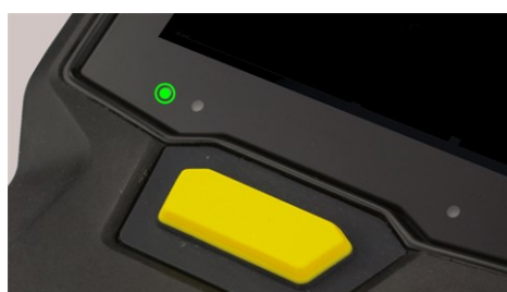
LED battery status indicator in sleep mode.
