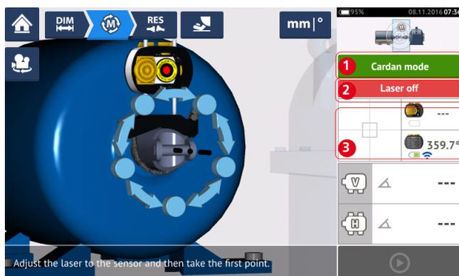
1 Tapping **1** reveals the three measurement procedures for cardan applications, as well access to both 'Tutorial' and 'Averaging'.
