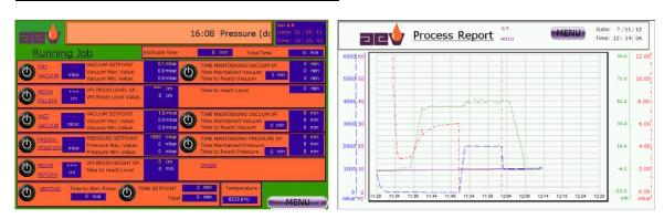
Process automation is carried out by a PLC which is installed at the control cabinet and allows the plant to operate the complete process automatically, semi-automatically or manually, allowing the operator to modify the main process parameters.
