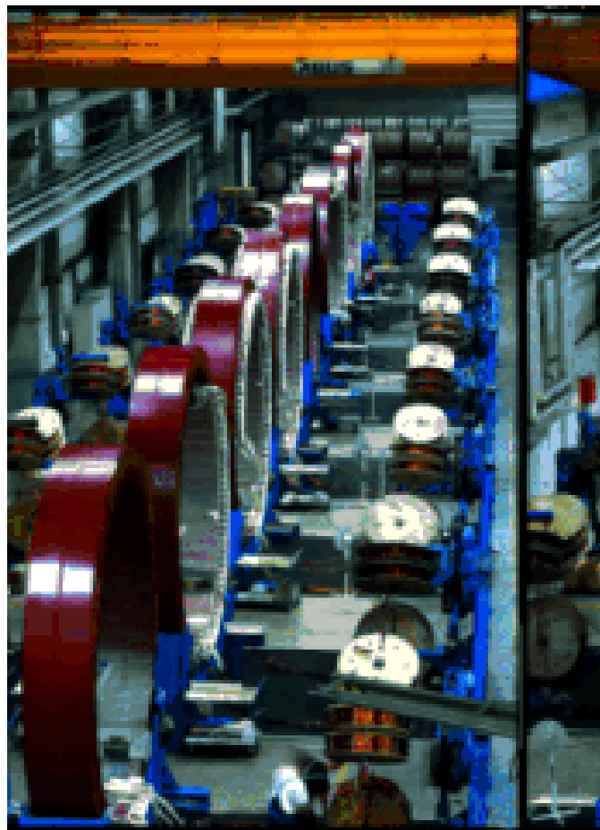
Fig. 22: Annular generators assembly line. Source: Enercon.
