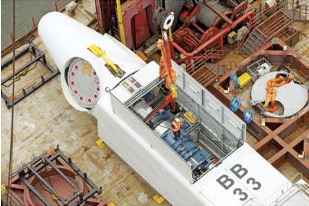
Fig. 11: Interior view of a Siemens wind turbine nacelle. Source: Siemens.
