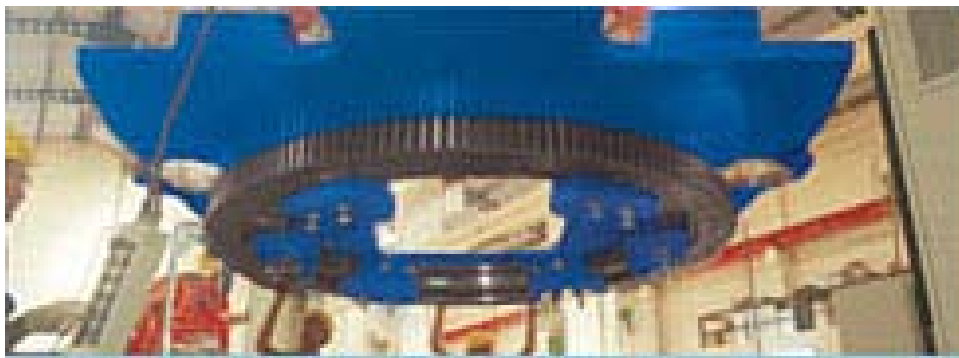
Fig. 6: The Suzlon 1.25 MW wind turbine generator yaw mechanism. Source: Suzlon.
