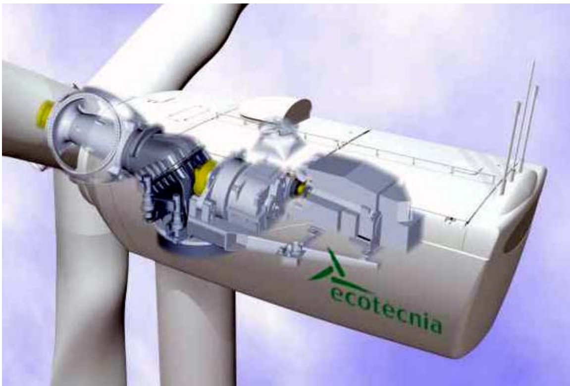
Fig. 63: The Ecotècnia rotor is directly supported by the structural tower. Source:
