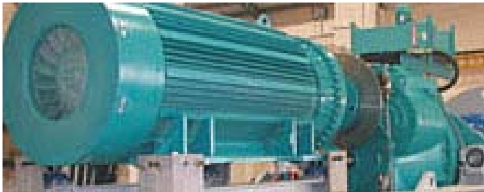
Fig.7: The Suzlon 1.25 MW electrical generator. Source: Suzlon.
