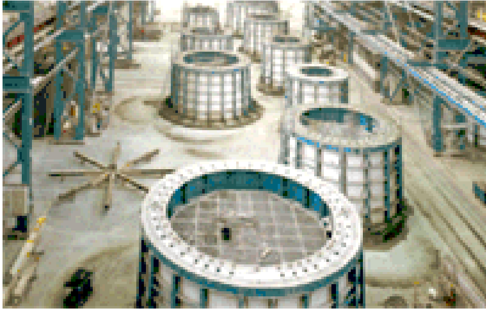
Fig. 39: Precast concrete tower sections.
