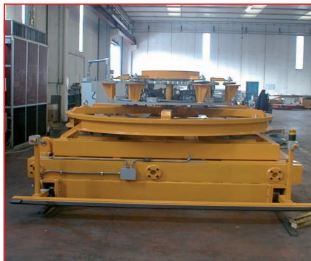
Masina Basculanta segment rachete Ariane Booster
