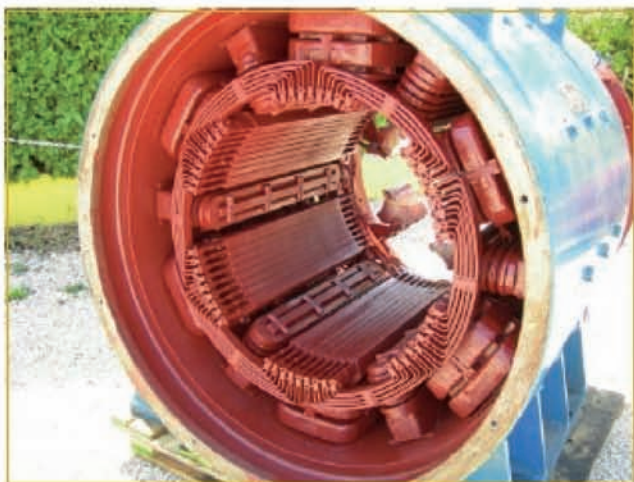
Motor C.C. 1500 Kw. 600 Volti dupa uscare in cuptor TEST CIRCULAR
