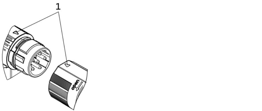
When connecting the cable connector to the motor connector, make sure that the aids to orientation (pos. 1) are facing each other. Only then trouble-free operation is ensured.
