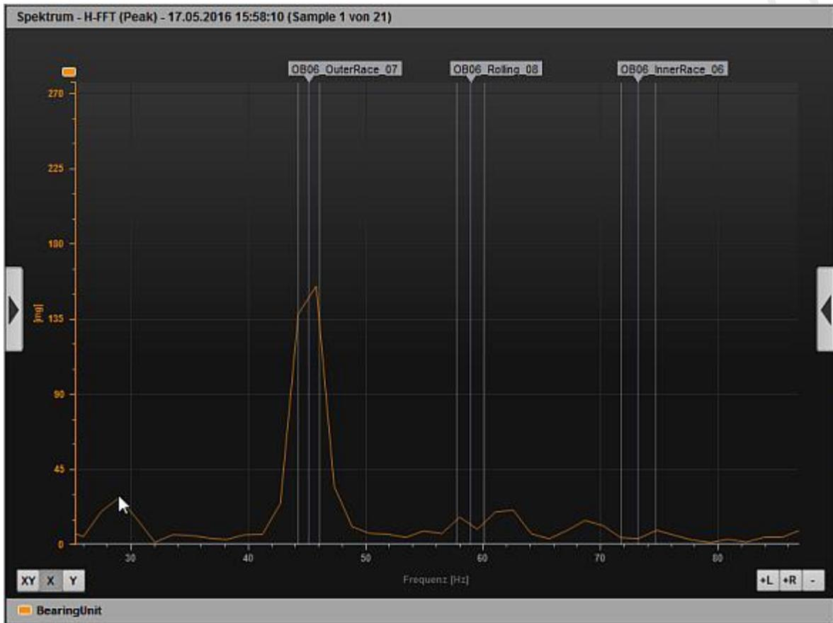
> The view clearly shows an imminent damage at the outer race of the bearing. Inner race and rolling element are free from damage.
