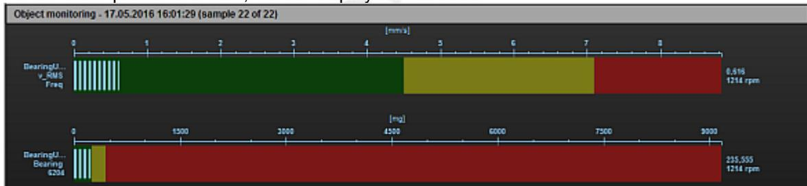
> The lower bar shows that the bearing is close to the warning alarm.
