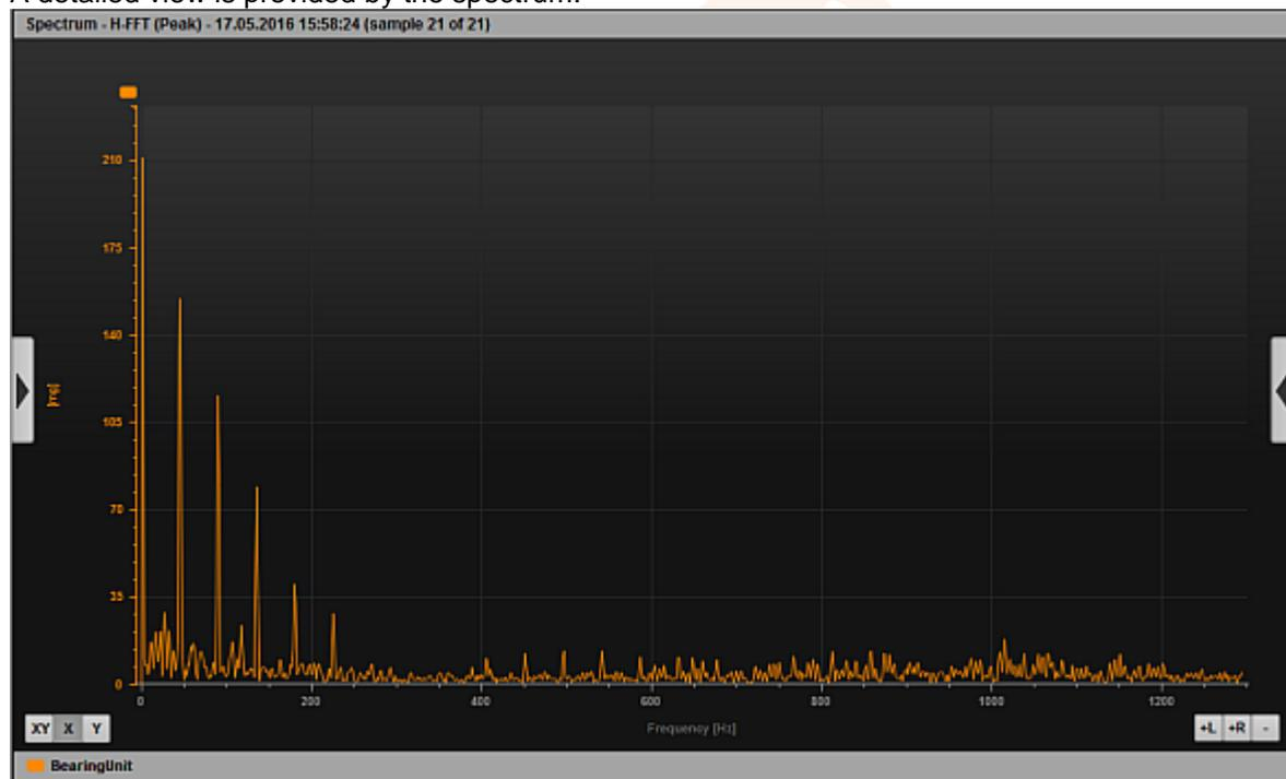
View: Measured data bearing damage (full screen)
