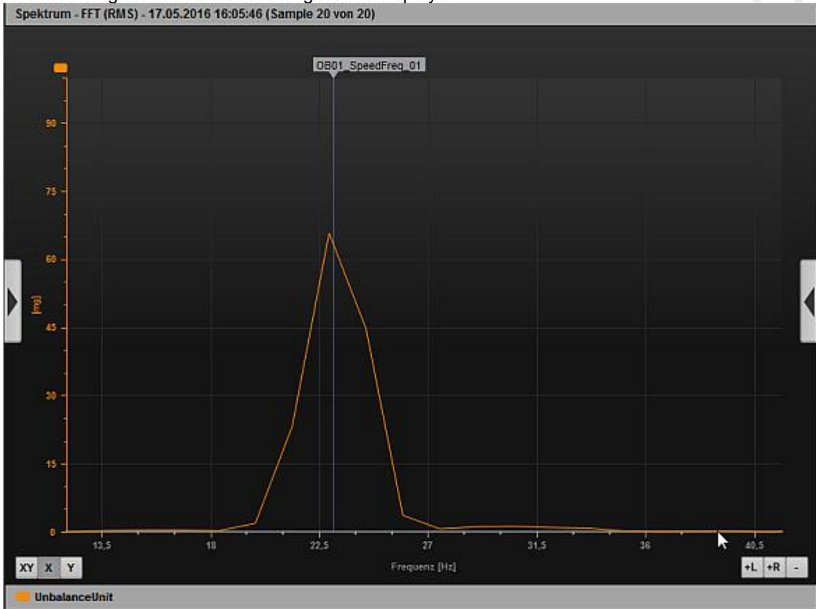
The bar graph shows that the unbalance is clearly in the warning alarm range:
