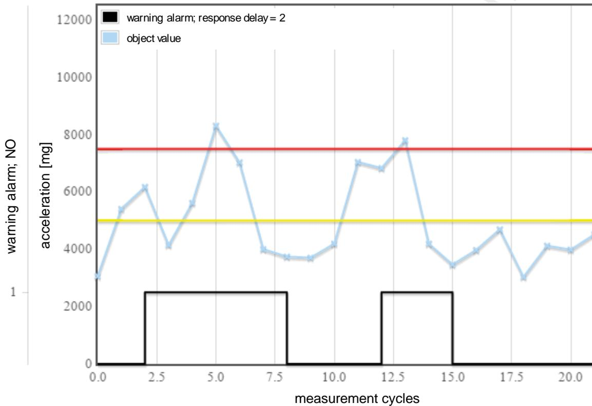
For example, during crash monitoring of a spindle, the response delay must be set to "1" to obtain the fastest possible crash alarm.
