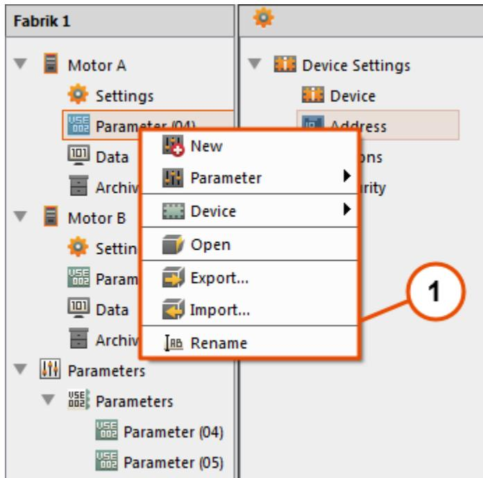
The context menu offers functions that are related to the selected element. For example, a new parameter can be created via the context menu of a parameter (1).
