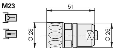
**Coupling (insulated):** Connecting element with outside thread; available with male or female contacts (see symbols).
