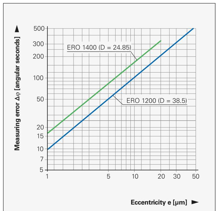
The following relationship exists between the eccentricity  $e$ , the mean graduation diameter  $D$  and the measuring error  $\Delta\varphi$  (see illustration below):
