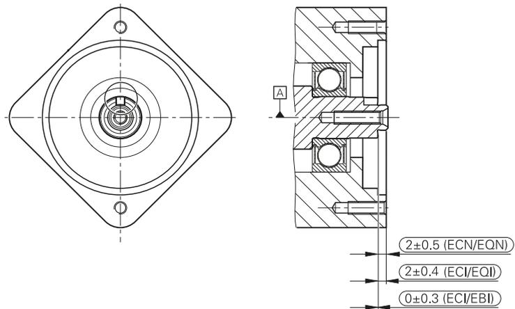
Some rotary encoders of the 1300 and ECN/EQN 400 series are mounting-compatible, and can therefore be mounted on identical seats. Slight differences, such as the anti-rotation element and the limited tolerance band of the inside diameter, must be taken into account.
