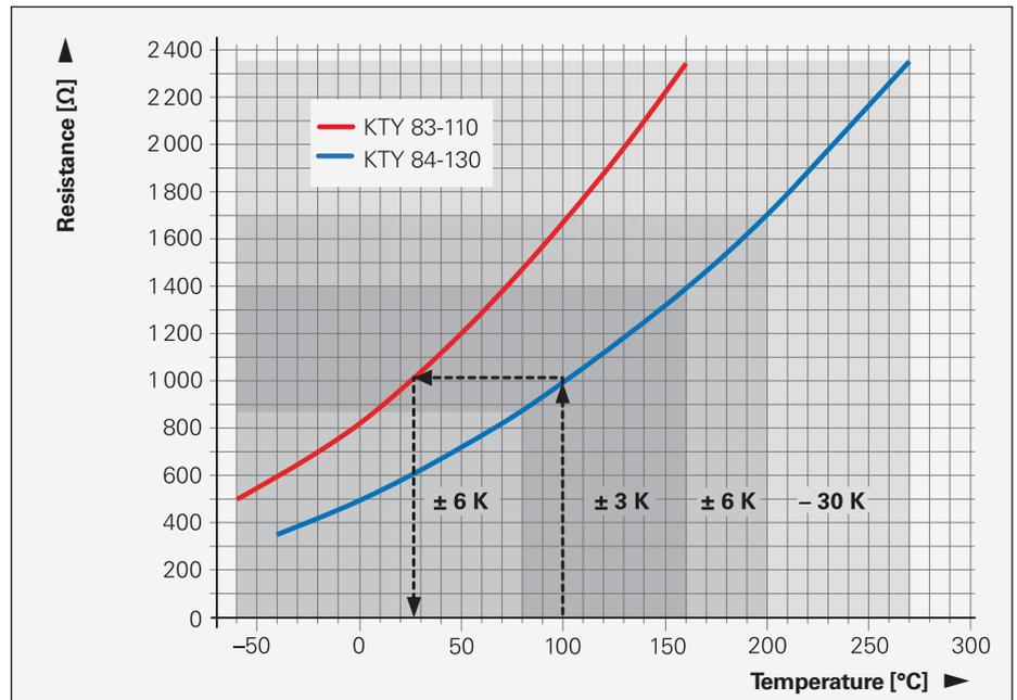
Relationship between the temperature and resistance value for KTY 84-130 and KTY 83-110 indicating the accuracy of temperature measurement and with a conversion example
