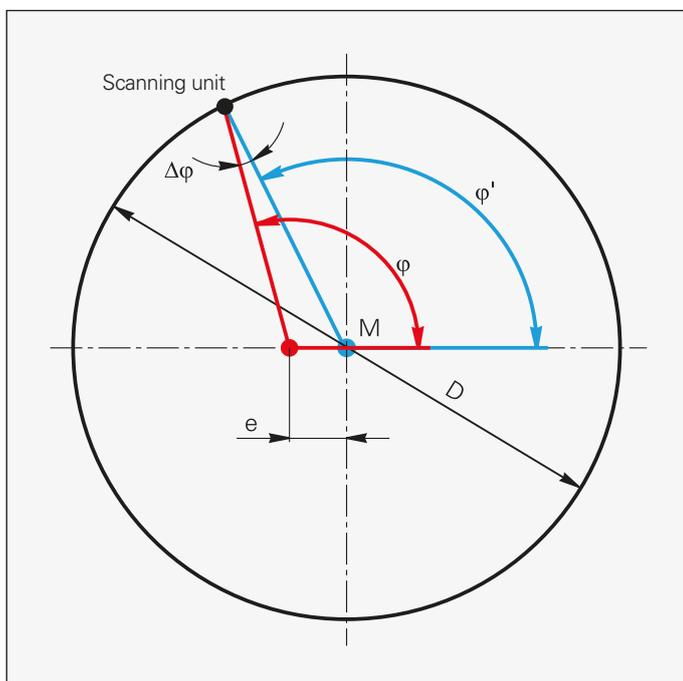
Measuring error  $\Delta\varphi$  as a function of the graduation centerline diameter  $D$  and the eccentricity  $e$
