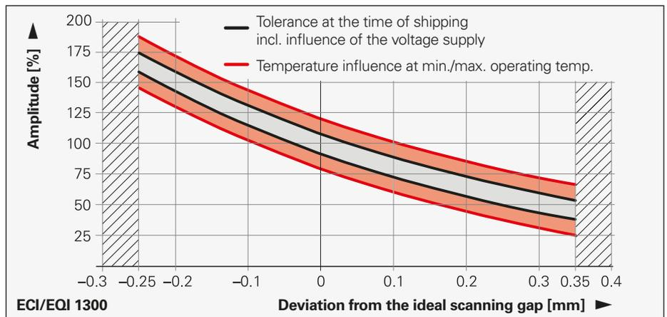
The **ECI/EQI 1300** inductive rotary encoders with EnDat01 are mechanically compatible with the ExN 1300 photoelectric encoders. The taper shaft (a bottomed hollow shaft is available as an alternative) is fastened with a central screw. The stator of the encoder is clamped by an axially tightened bolt in the location hole. The scanning gap between rotor and stator must be set during mounting.
