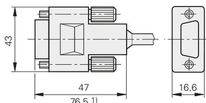
1) Interface electronics are integrated in the connector
