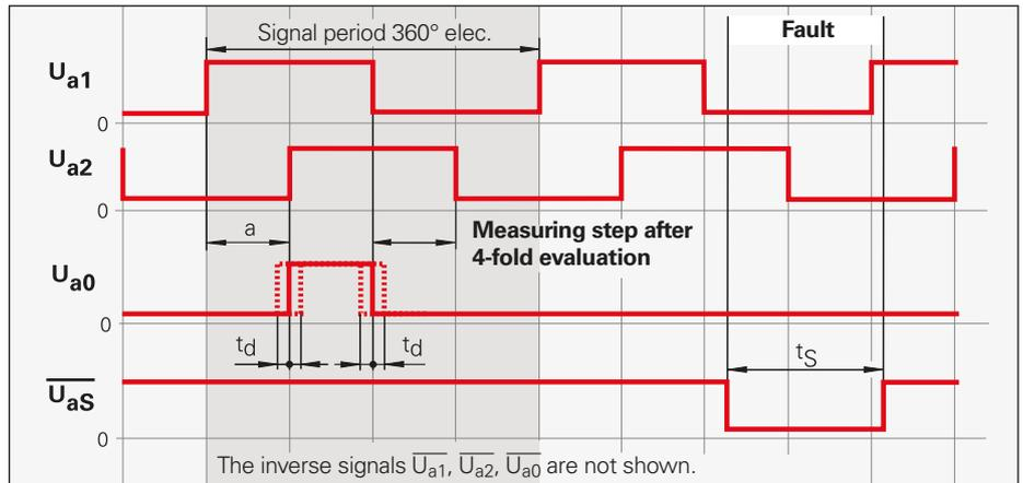
The distance between two successive edges of the incremental signals  $U_{a1}$  and  $U_{a2}$  through 1-fold, 2-fold or 4-fold evaluation is one **measuring step**.
