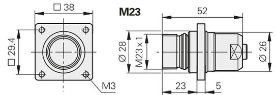
**Flange socket:** With external thread; permanently mounted on a housing, available with male or female contacts.
