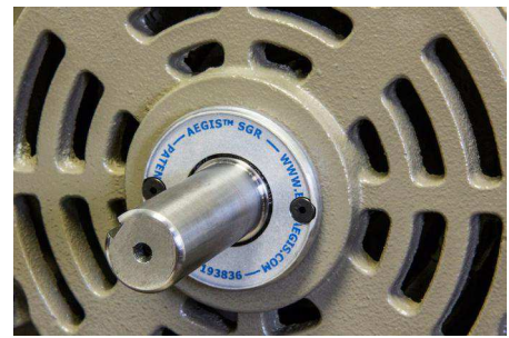
External Installation on Motor Bracket
