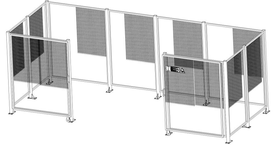
Electro-welded net square grid 22x100 wire  $\phi 3$
