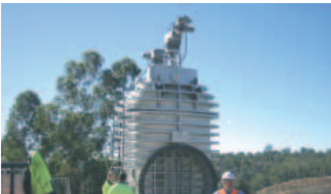
Gate valves with mounted AUMA actuator for a dam project in Australia before installation.
