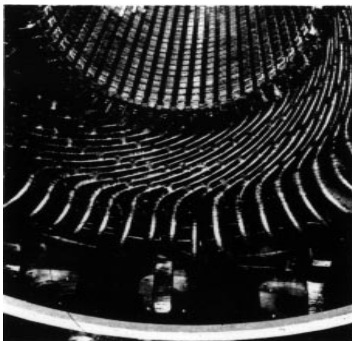
Figure 5. Stator Winding End Turns and Connections for a Two-Pole, Spring-Bar Mounted Hydrogen-Cooled Turbine-Generator
