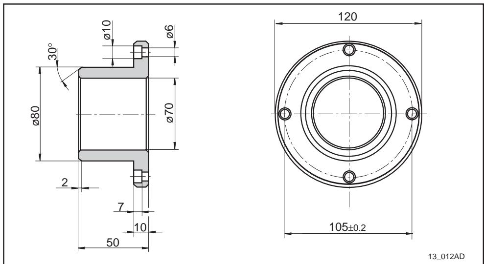
Fig. 13.1: Dimensions of blower base for 2AD132/134
