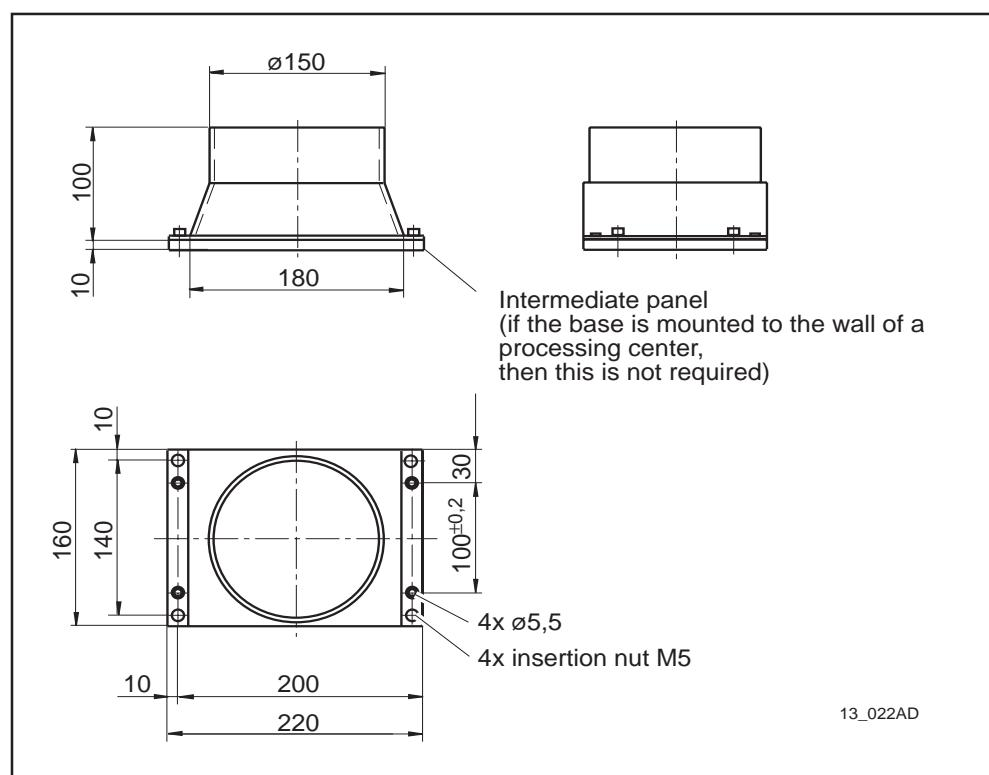
Fig. 13.2: Dimensions of blower base for 2AD160/164
