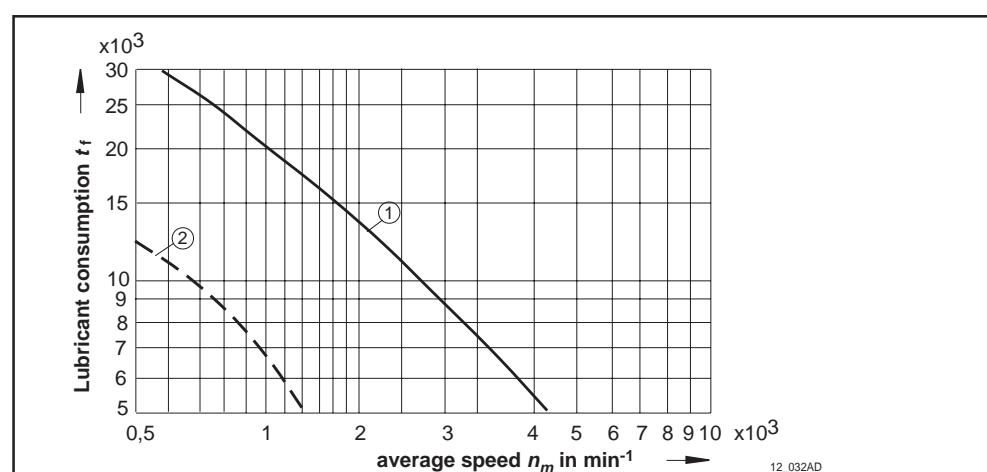
Fig. 12.3: Lubricant consumption 2AD225
