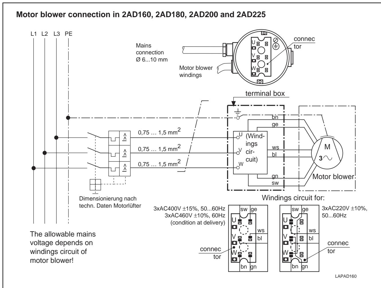
Fig. 14.17: Terminal diagrams for motor blower of 2AD160/-180/-200/-225
