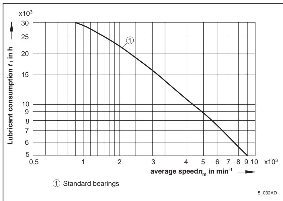
Fig. 5.3: Lubricant consumption duration 2AD104
