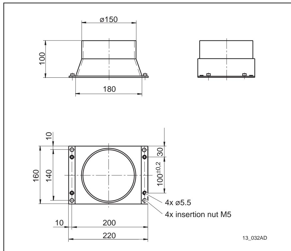
Fig. 13.3: Dimensions of blower base for 2AD180
