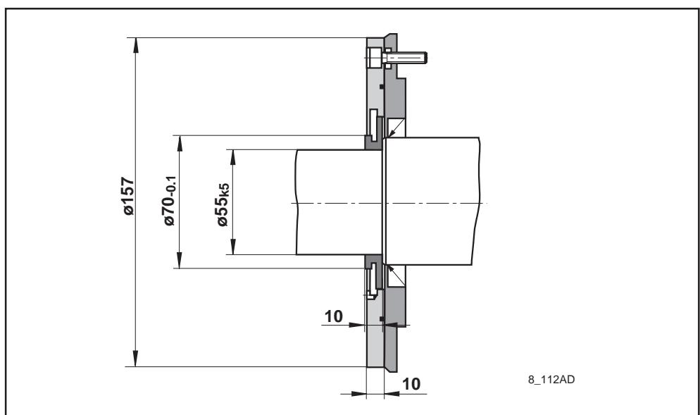
Fig. 8.11: 2AD160 with accessories mounted M02 2AD160/164 (Labyrinth seal)
