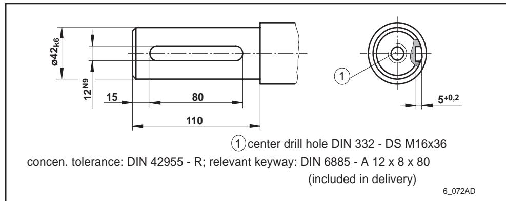
Fig. 6.7: Output shaft with key for 2AD132
