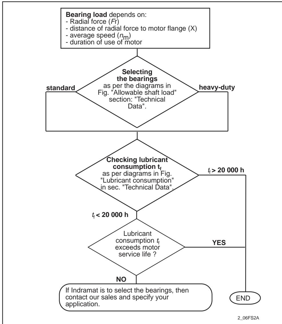
Fig. 2.6: The sequence for determining bearing assembly
