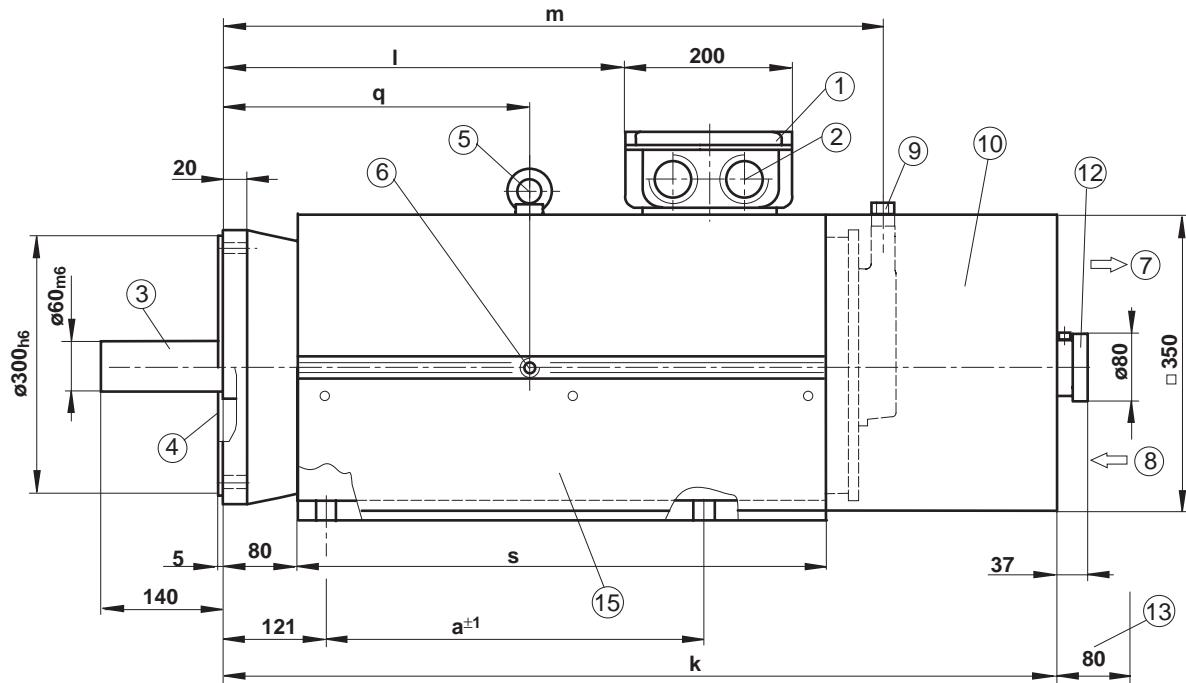
**Motor with radial blower and feedback type 3, B35**
