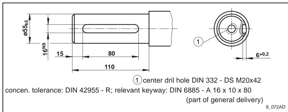
Fig. 8.7: Output shaft with key for 2AD160
