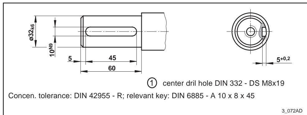
Fig. 3.7: Output shaft with key for 2AD100
