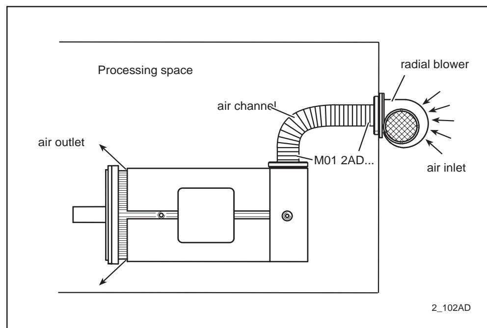
Fig. 2.10: Motor cooling via air channel - possible solution
