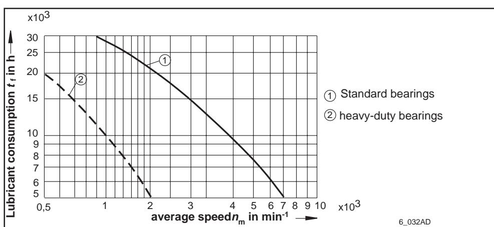
Fig. 6.3: Lubricant consumption duration 2AD132
