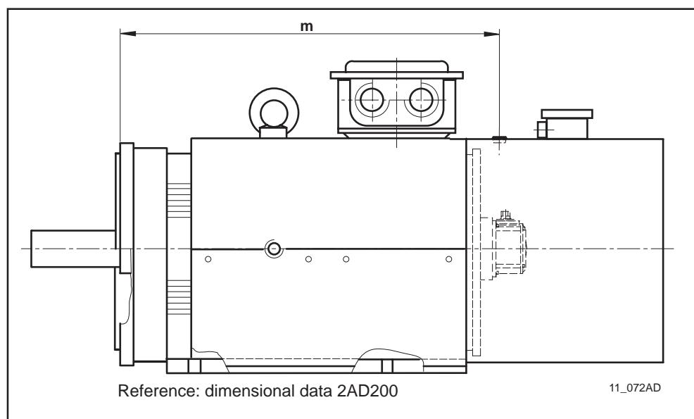
Fig. 11.7: 2AD200 with feedback types 6, 7
