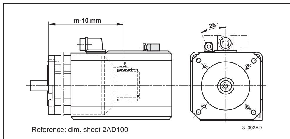
Fig. 3.9: 2AD100 with feedback types 6, 7
