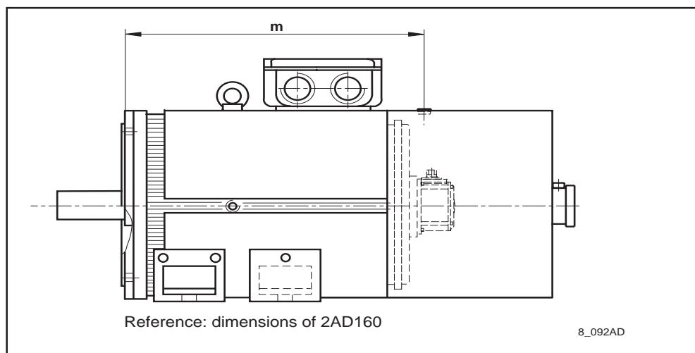
Fig. 8.9: 2AD160 with feedback types 6, 7
