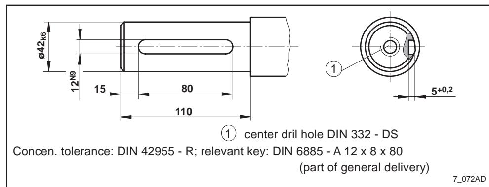
Fig. 7.7: Output shaft with key for 2AD134
