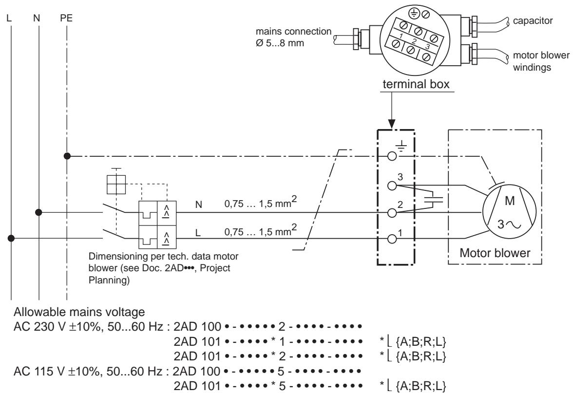
**Axial blower connection in 2AD101(conn.) and 2AD104 (air flow A=>B)**
