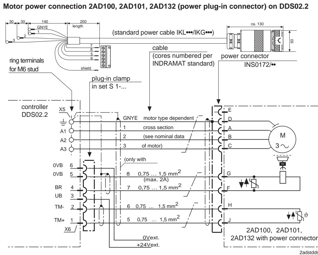
Fig. 14.2: Terminal diagram for motors with power plug-in connector on DDS02.2
