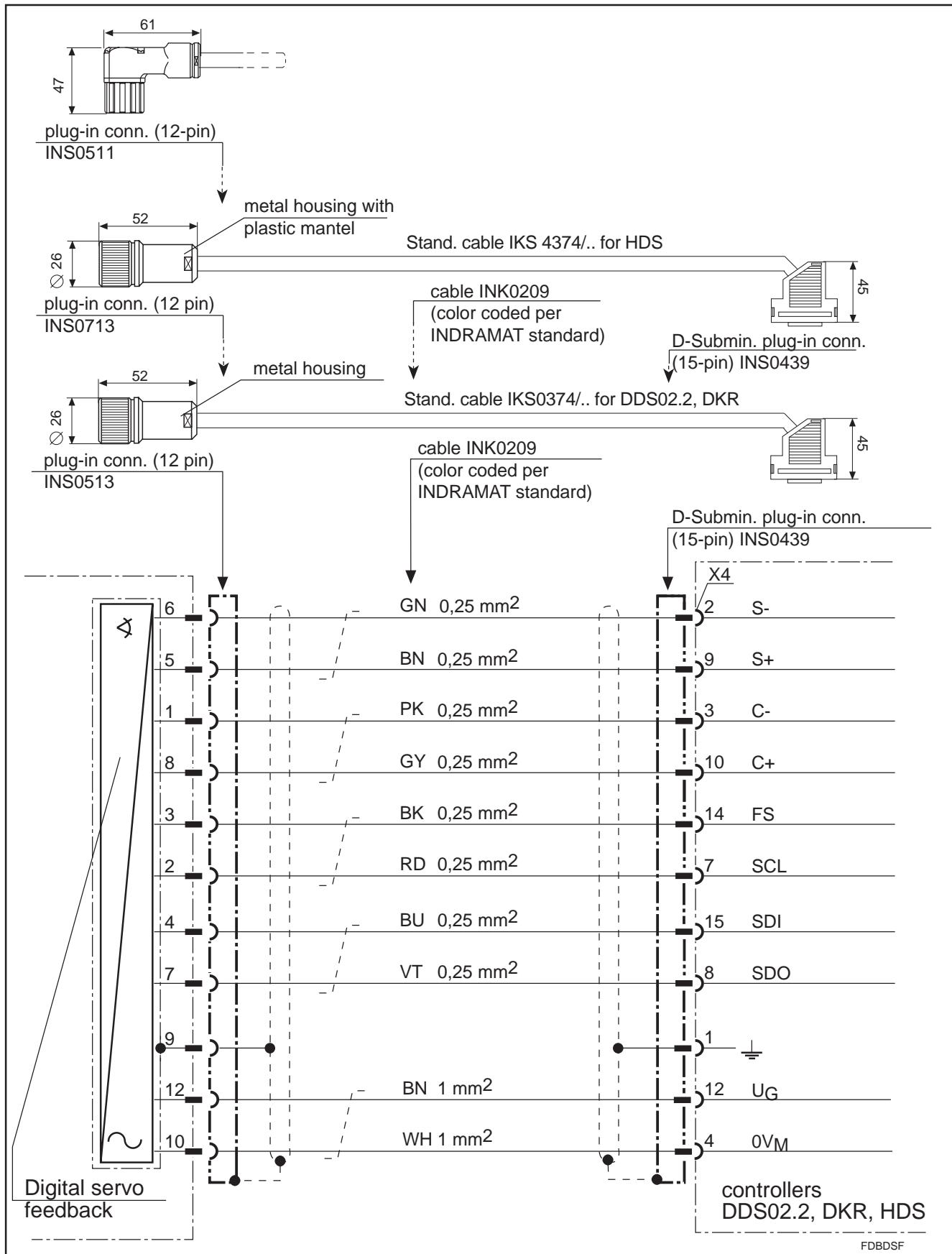
Fig. 14.20: Terminal diagrams for high-resolution motor feedback ("6"; "7") on DDS02.2/DKR/HDS
