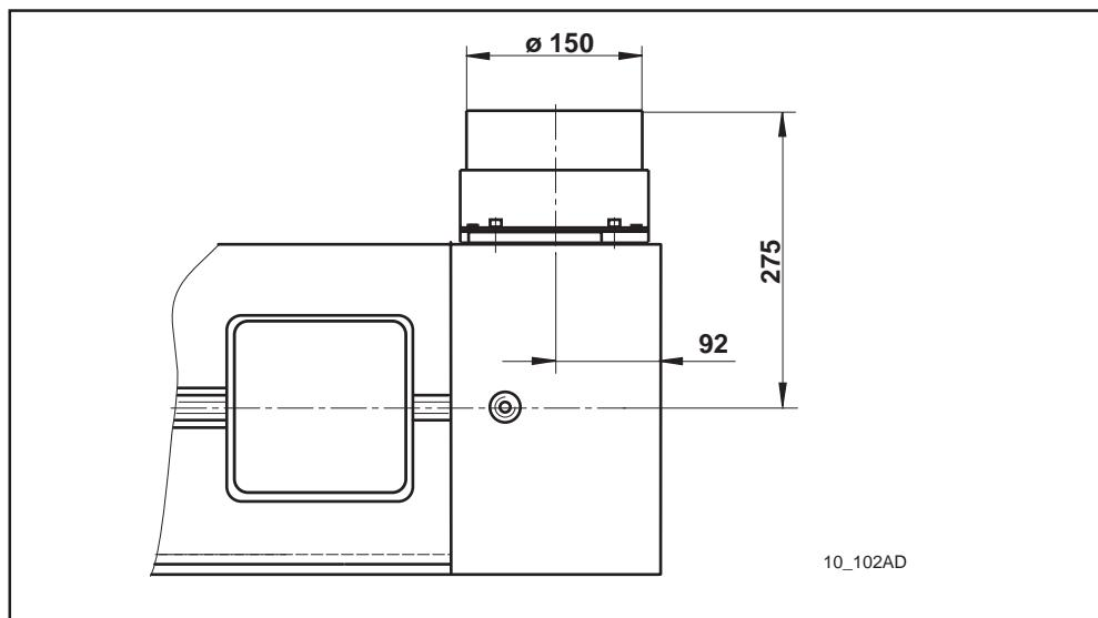
Fig. 10.10.: 2AD180 with mounted accessories - M01 2AD180 (blower base)
