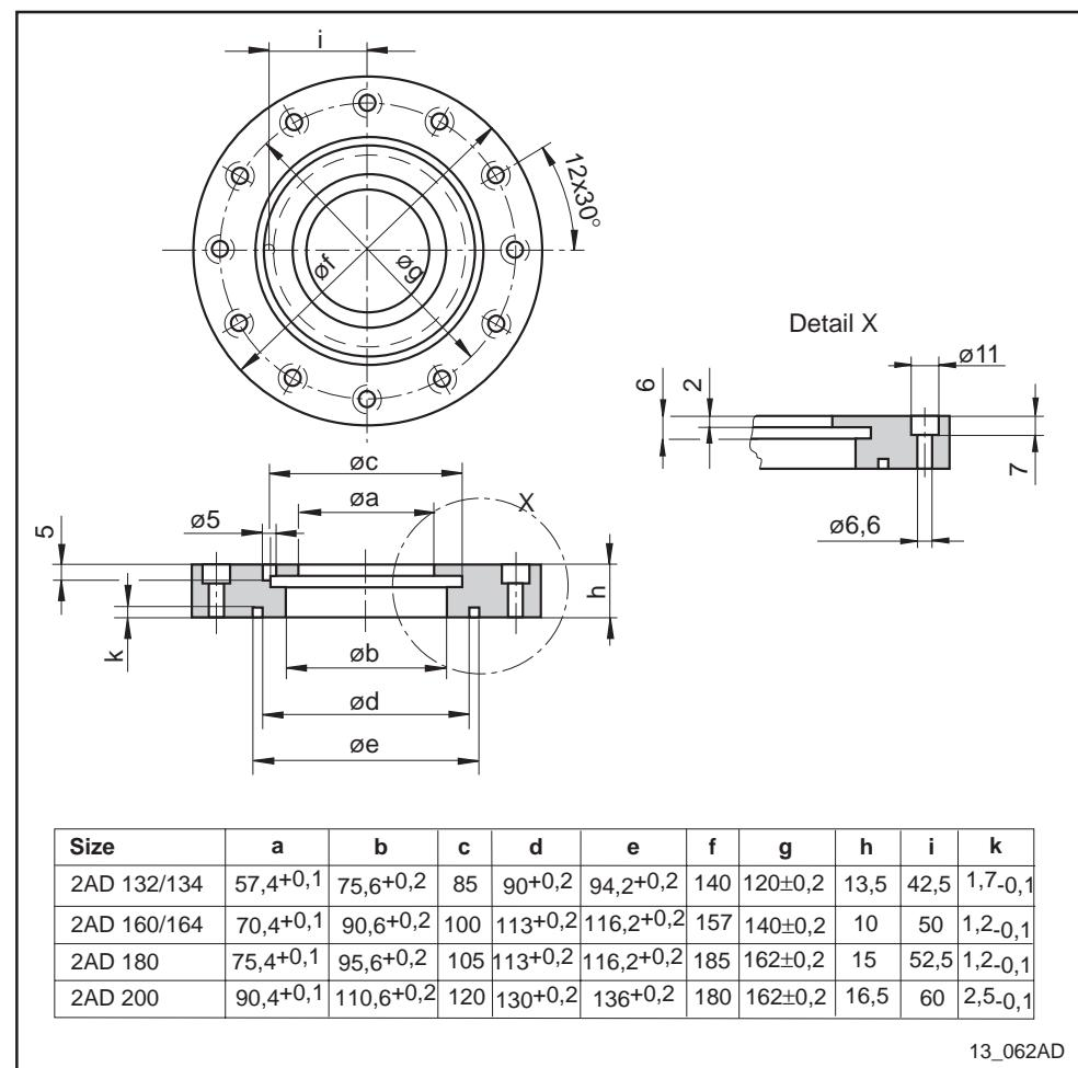
Fig. 13.6: Flange of the mechanical accessories M02 2AD...
