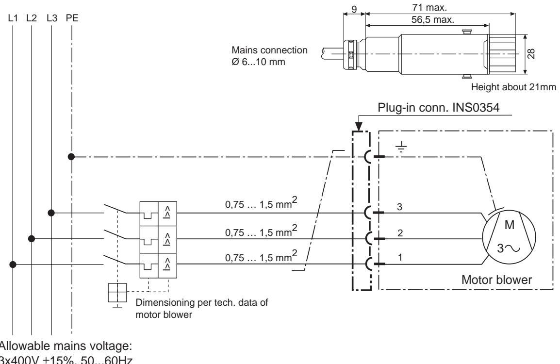
Fig. 14.16: Terminal diagrams for motor blower of 2AD132/-134/-164
