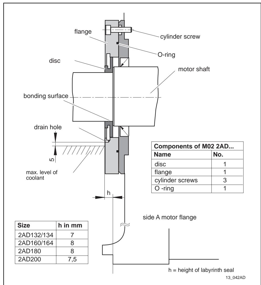
Fig. 13.4: Construction principle of the labyrinth seal
