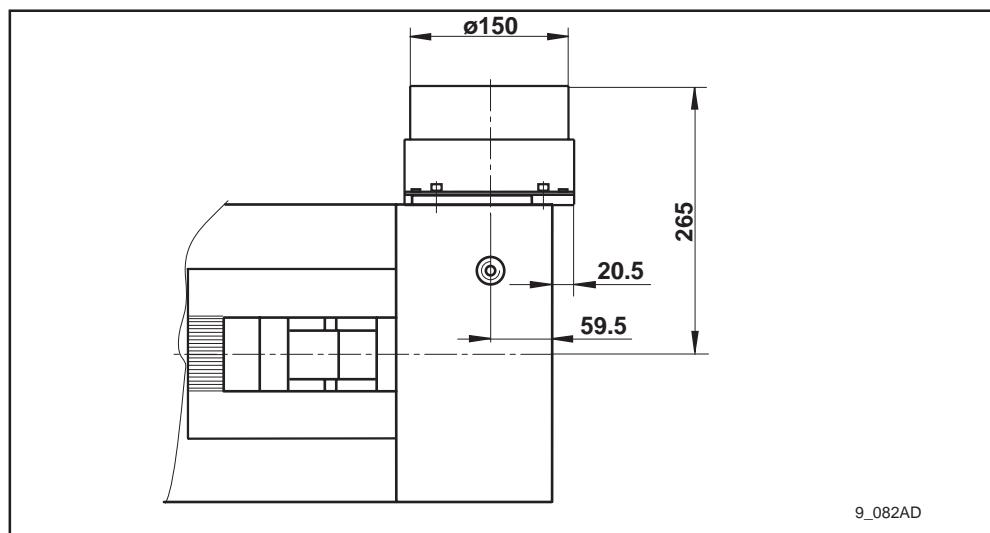
Fig. 9.8: 2AD164 with mounted accessories - M01 2AD160/164 (blower base)
