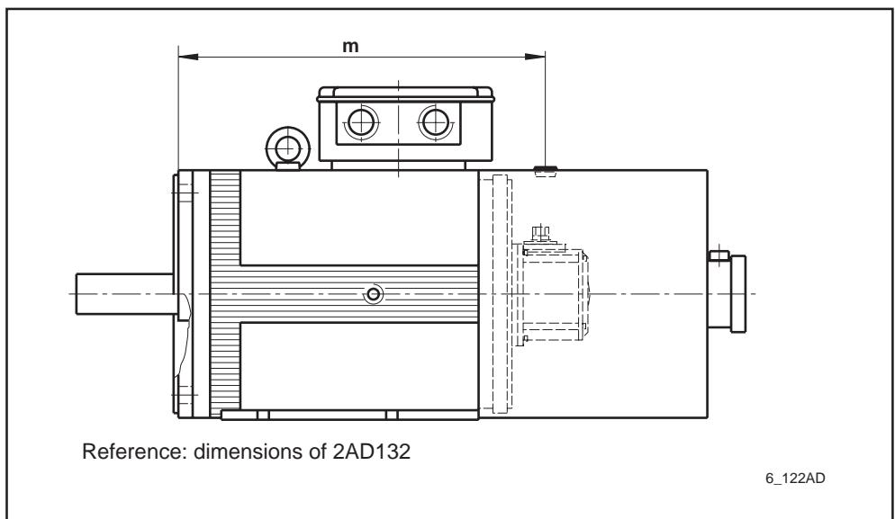
Fig. 6.12: 2AD132 with feedback types 6, 7
