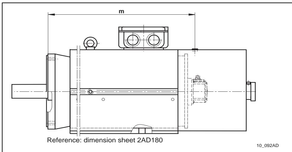
Fig. 10.9.: 2AD180 with feedback types 6, 7
