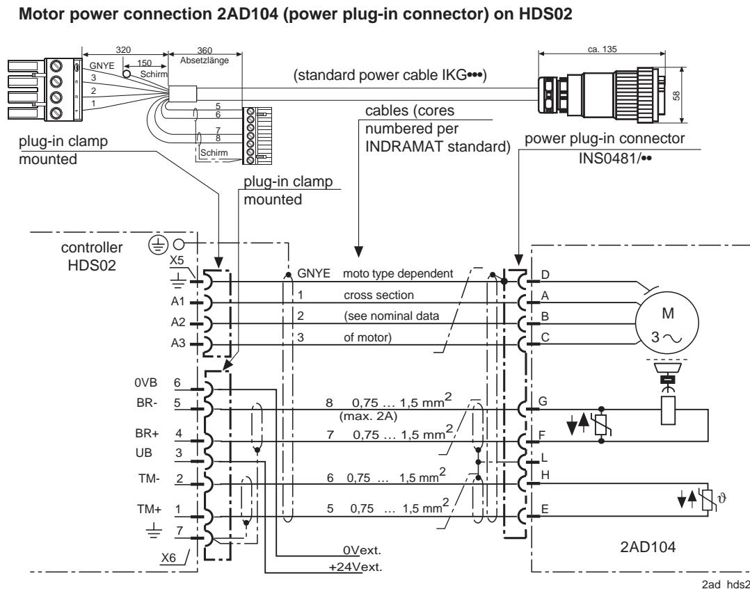
Fig. 14.3: Terminal diagram for motors with power plug-in connector on HDS02
