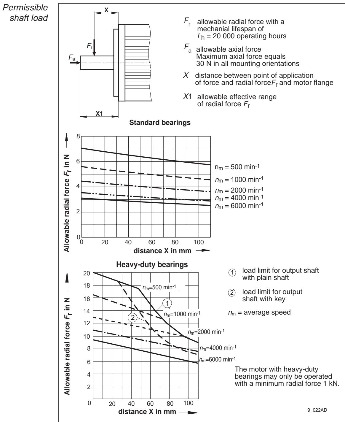
Fig. 9.2: Permissible shaft load 2AD164
