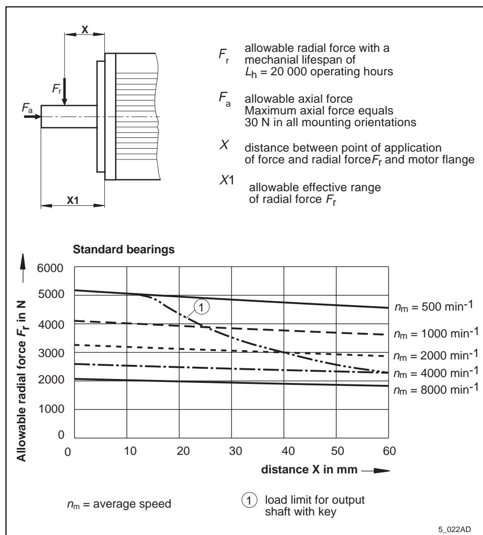
Fig. 5.2: Permissible shaft load 2AD104
