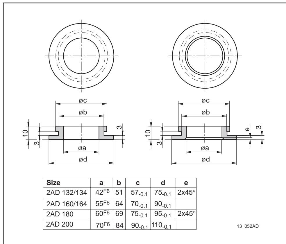
Fig. 13.5: Disc of mechanical accessories M02 2AD...
