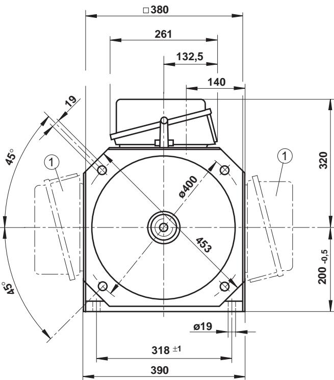
① power connection; arrangement selectable, can be turned by 90°, in terms of output direction of power connection
