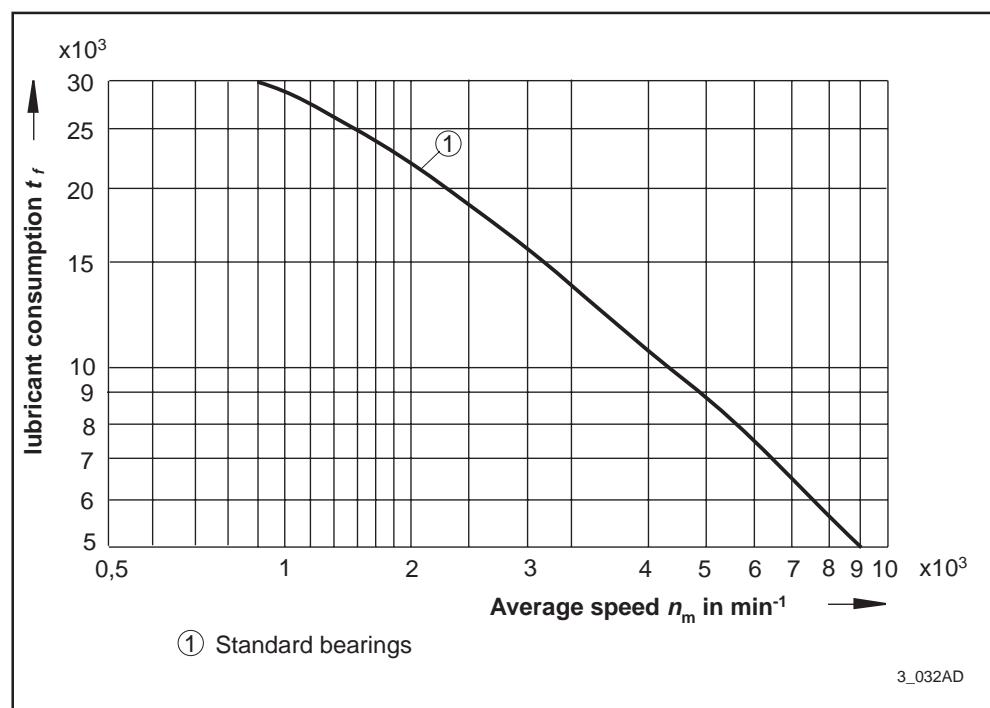
Fig. 3.3: Lubricant consumption duration 2AD100
