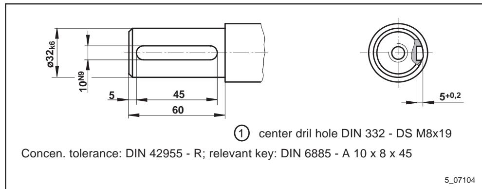
Fig. 5.7: Output shaft with key for 2AD104
