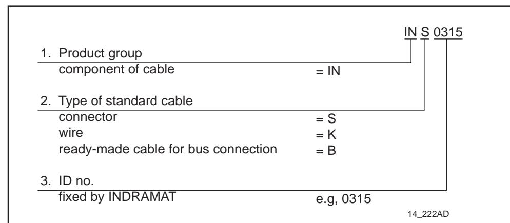
Fig. 14.22: Type designation of components of standard cables
