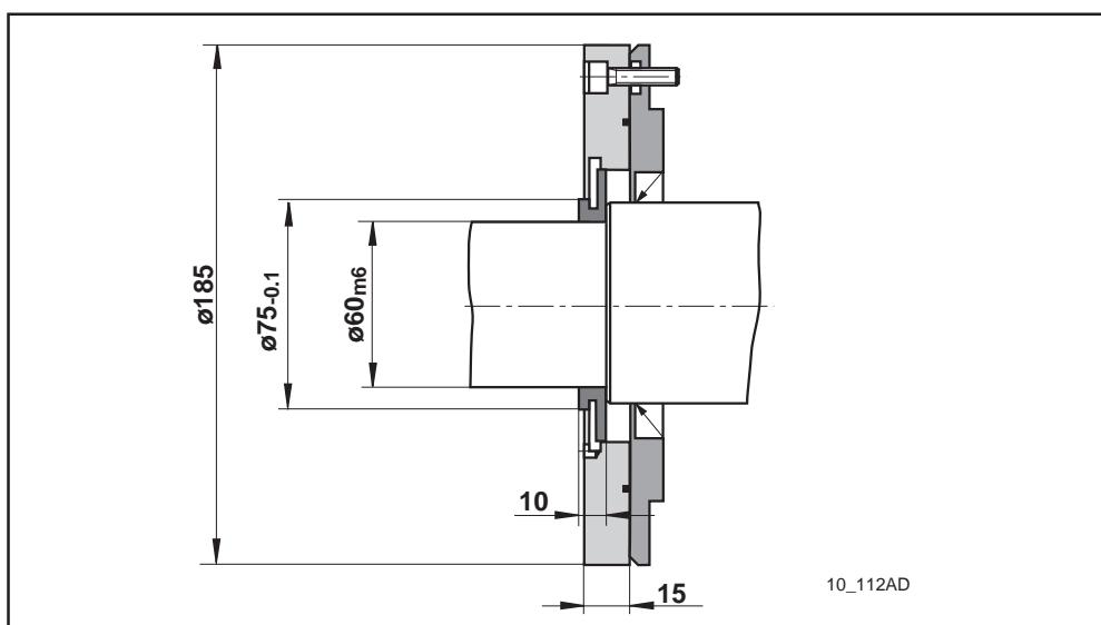
Fig. 10.11: 2AD180 with mounted accessories - M02 2AD180 (labyrinth seal)
