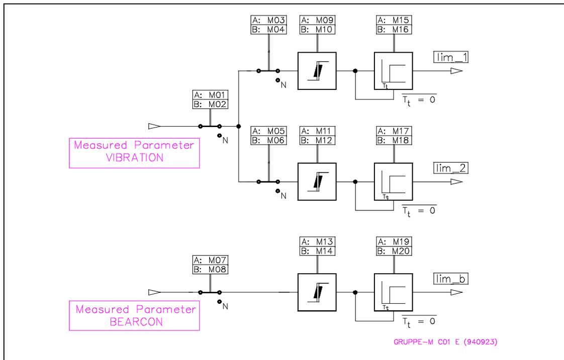
Fig. 5 - 6 : Parameter Group M, Limit Value Configuration
