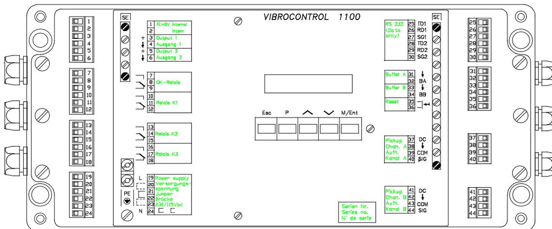
Figure 1-1: Top view of a VIBROCONTROL 1100 with cover removed
