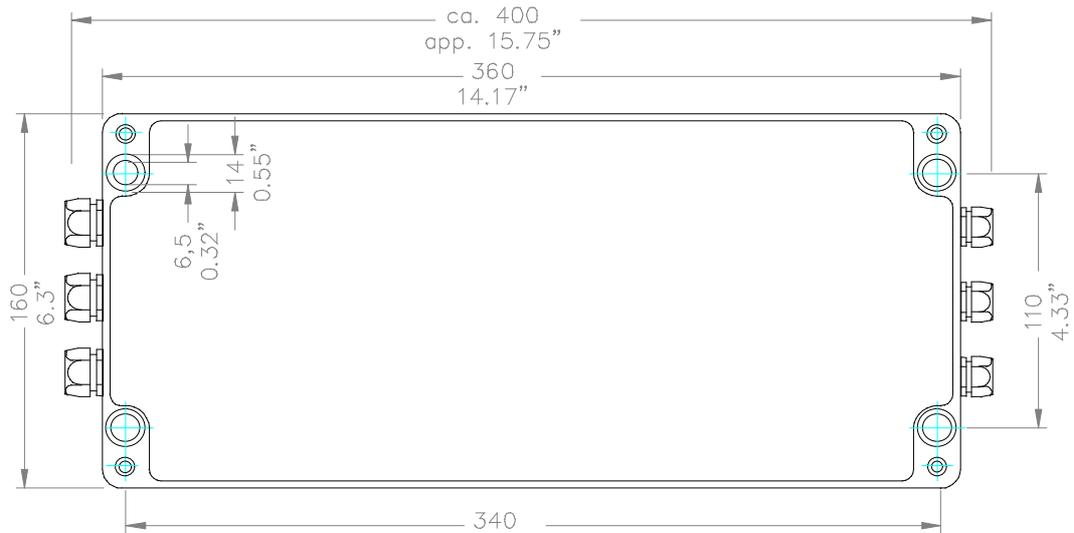
Figure 2-1: Housing Dimensions
