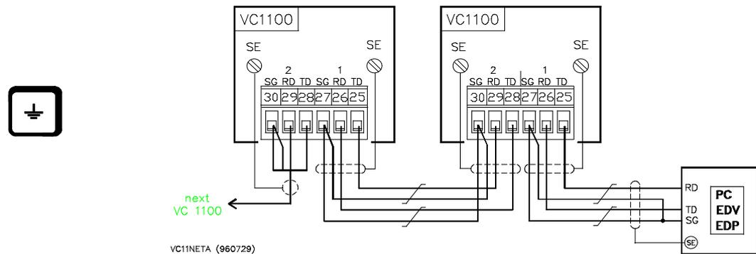
Fig. 3 - 11: Interfacing a HOST with several VC-1100's
