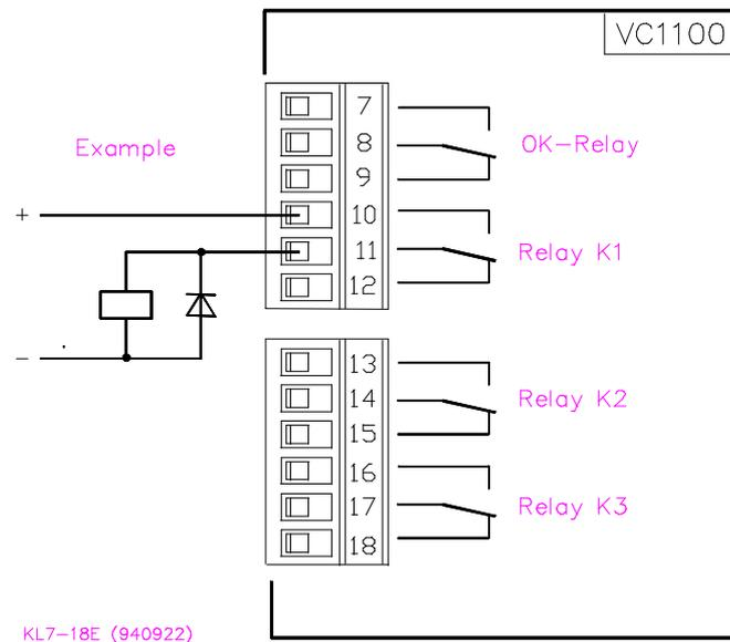
Fig. 3 - 5 : Connecting the-Relays
