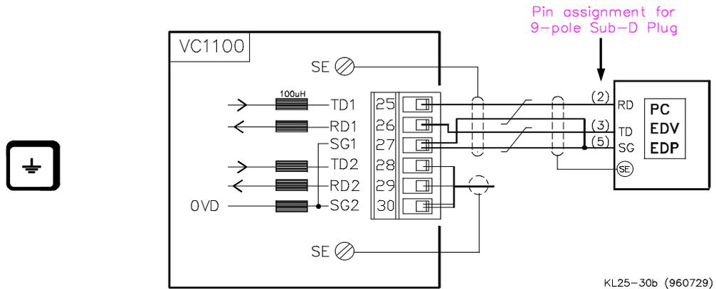
Fig. 3 - 9: Interfacing a HOST with one VC-1100
