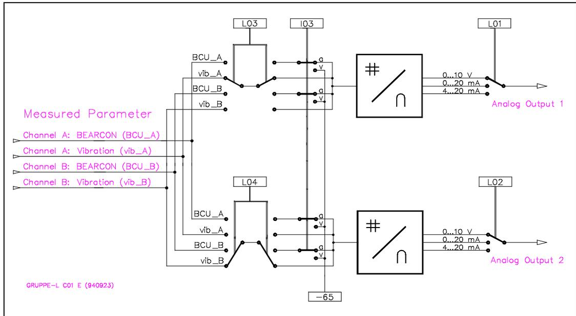
Fig. 5 - 5: Parameter Group L, Analog Outputs
