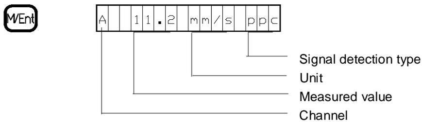
The display shows vibration level of channel A. A flashing display indicates a limit value was exceeded.
