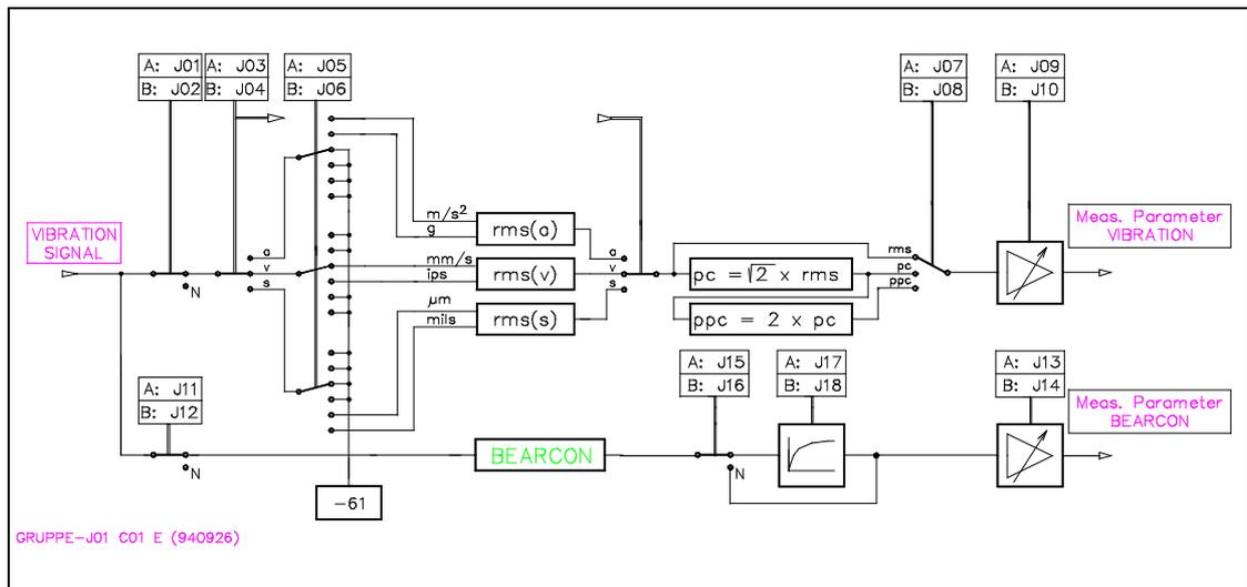
Fig. 5 - 3: Parameter Group J, Signal Detection Type
