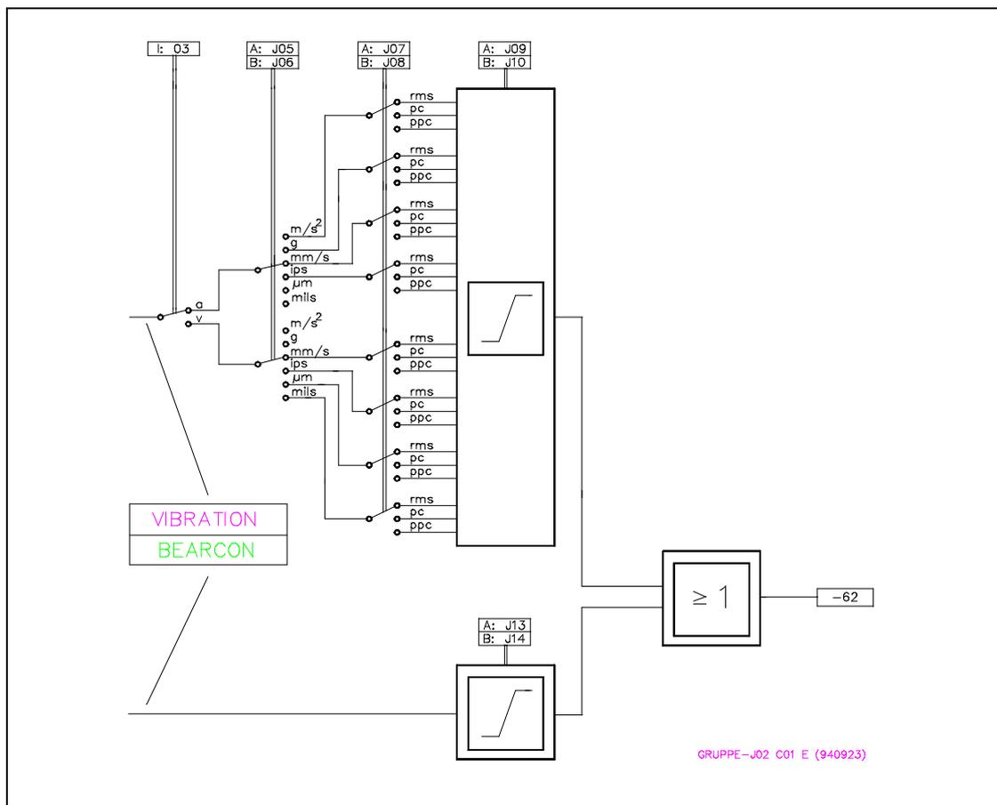
Fig. 5 - 4: Parameter Group J, Signal Detection Type
