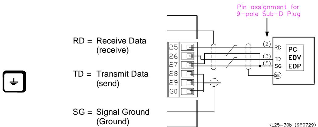
Fig. 3 - 10: Interfacing a HOST with one VC 1100
