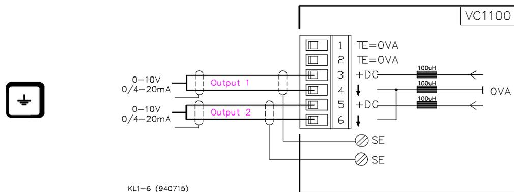
Fig. 3 - 7: Connecting Analog Outputs
