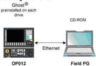
For backup and restore, a backup computer is connected to the PC via the Ethernet interface. Ghost<sup>®</sup> is installed as standard on all PCU hard disks and is also entered in the standard service menu. The Ghost<sup>®</sup> is started here using the appropriate menu items. Data backup or restore runs without
