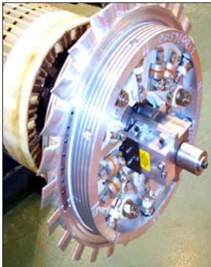
Fig.1 Transmitter fitted to generator rotor
