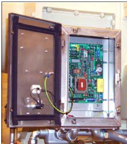
Fig.2 Receiver in IP66 enclosure for generator mounting
