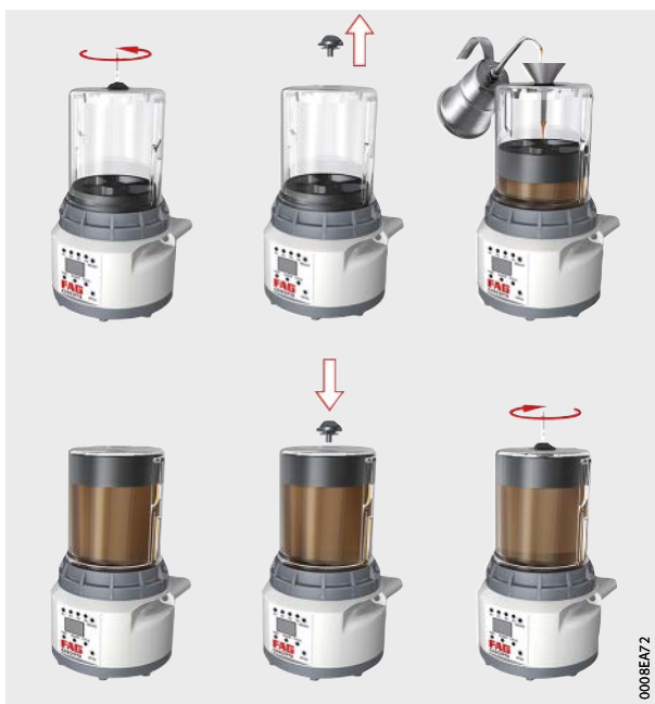
Figure 60 Refilling the oil reservoir
