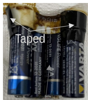
Non-original battery cells
