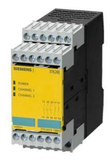
SIRIUS SAFETY RELAY WITH RELAY RELEASE CIRCUITS (RC), DC 24V, 45.0MM, SCREW TERMINAL, RC INSTANT.: 3NO, RC DELAYED: 0NO, MK: 2NC, AUTOSTART / MONITORED START, BASIC DEVICE, MAX. ACHIEVABLE SIL: 3, PL: E
