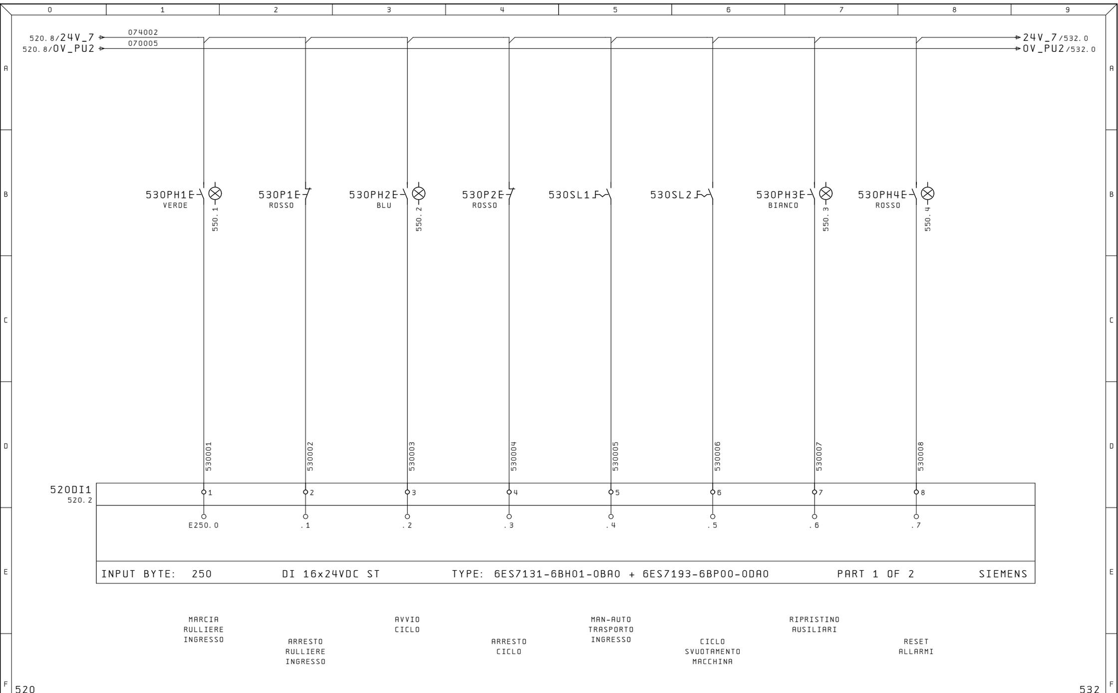
INPUT BYTE: 250      DI 16x24VDC ST      TYPE: 6ES7131-6BH01-0BA0 + 6ES7193-6BP00-0DA0      PART 1 OF 2      SIEMENS
