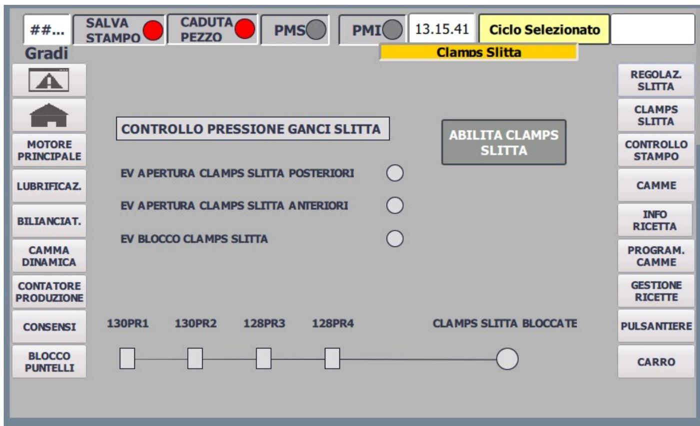
NELLA PAGINA CLAMPS SLITTA VISUALIZZIAMO I FINECORSA DELLE CLAMPS E LO STATO DELLE ELETTROVALVOLE (CHIUSE/APERTE) DELLE STESSE.
