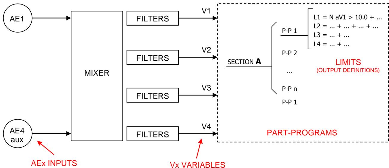
Starting from the AEx sensors connected to the inputs of the card (connectors D8, D5) it is necessary to define the Vx variables to perform the process control.
