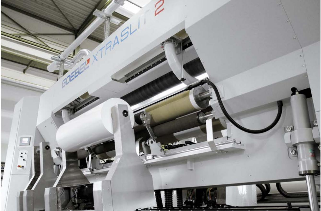
The GOEBEL XTRASLIT 2 is an innovative slitter rewriter and sets standards for highly productive processing of paper, film and foil, and flexible packaging materials.
