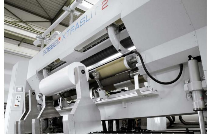
The GOEBEL XTRASLIT 2 is an innovative slitter rewinder and sets standards for highly productive processing of paper, film and foil, and flexible packaging materials.
