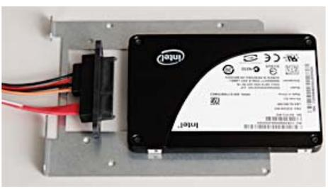
A photograph of the Intel SSD removed from the mount. The SSD is a 2.5-inch drive with a black top and a white label. The label includes the Intel logo, 'SSD', '160GB', and other technical specifications. The SATA connector is visible on the left side. |
