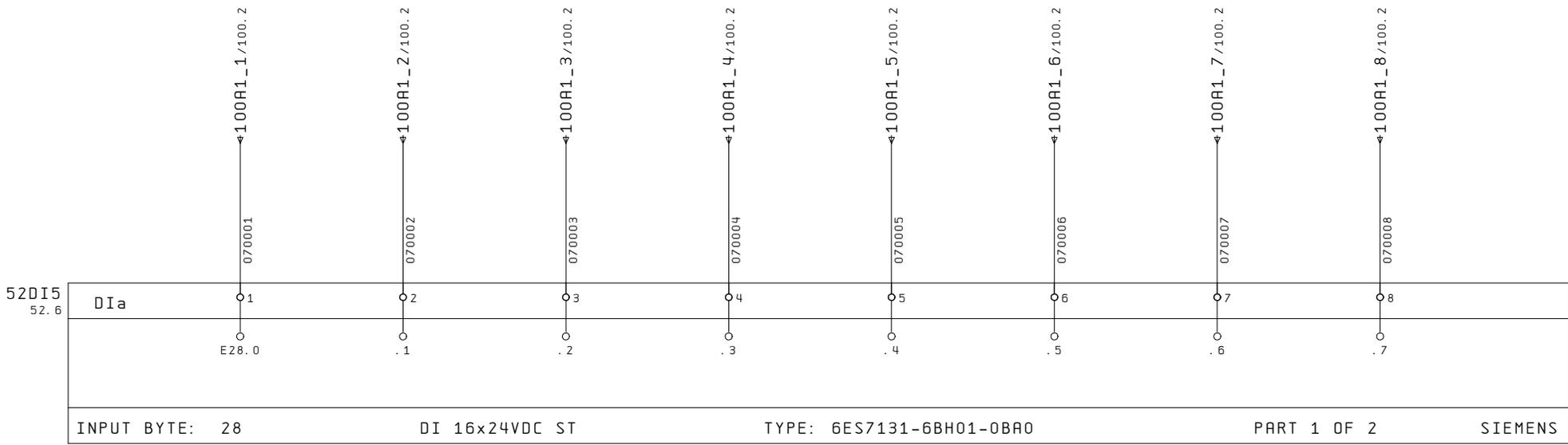
INPUT BYTE: 28      DI 16x24VDC ST      TYPE: 6ES7131-6BH01-0BA0      PART 1 OF 2      SIEMENS
