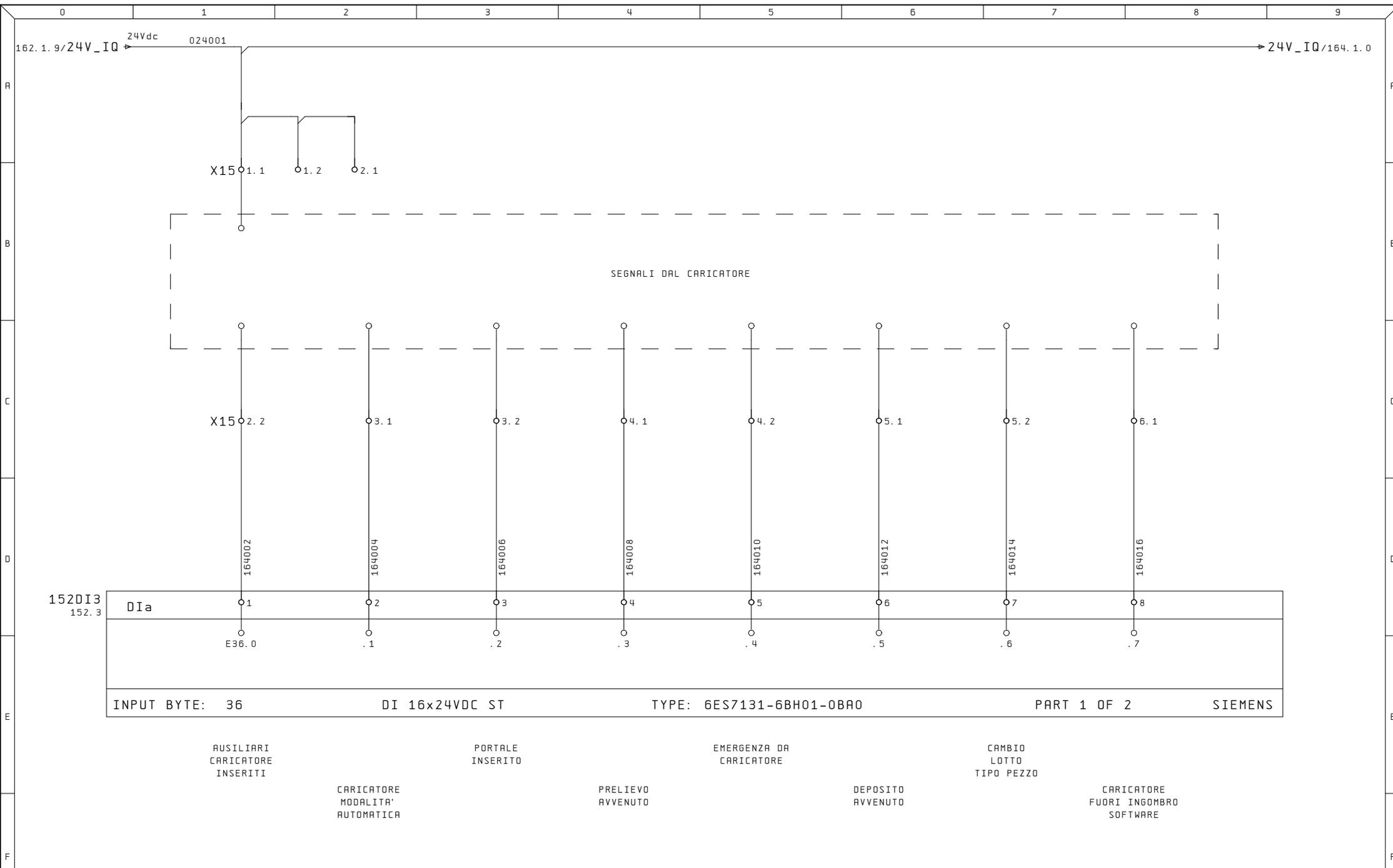
INPUT BYTE: 36      DI 16x24VDC ST      TYPE: 6ES7131-6BH01-0BA0      PART 1 OF 2      SIEMENS
