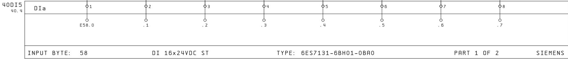
INPUT BYTE: 58      DI 16x24VDC ST      TYPE: 6ES7131-6BH01-0BRA0      PART 1 OF 2      SIEMENS
