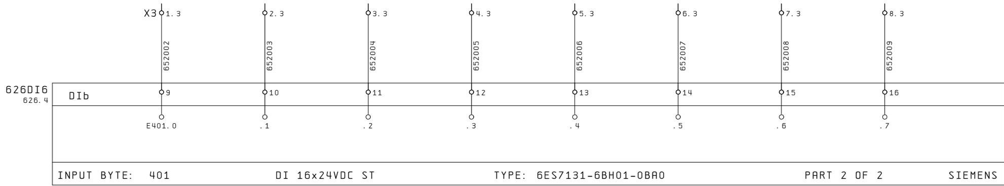
INPUT BYTE: 401                      DI 16x24VDC ST                      TYPE: 6ES7131-6BH01-0BR0                      PART 2 OF 2                      SIEMENS
