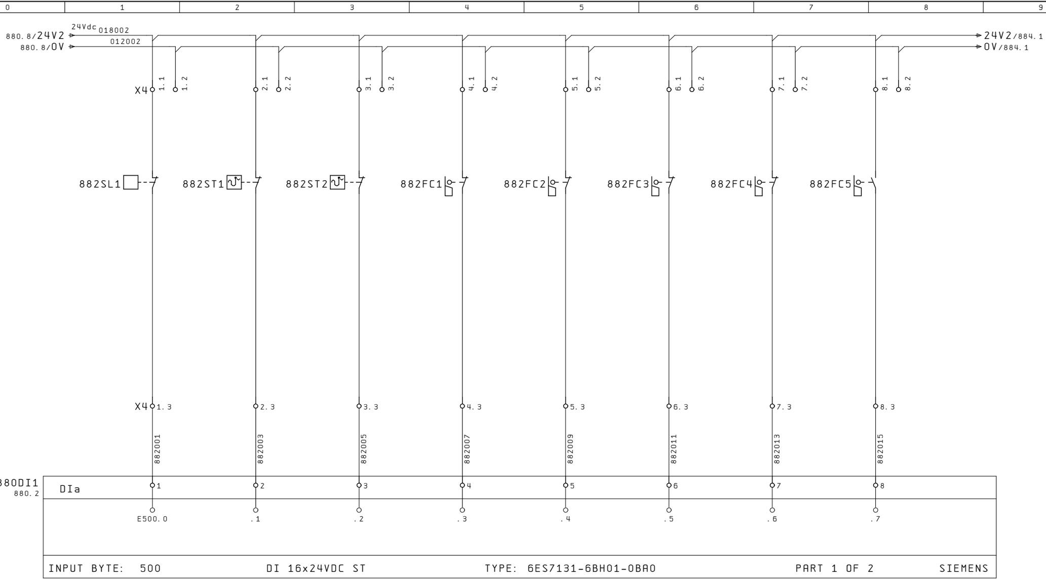
INPUT BYTE: 500      DI 16x24VDC ST      TYPE: 6ES7131-6BH01-0BA0      PART 1 OF 2      SIEMENS
