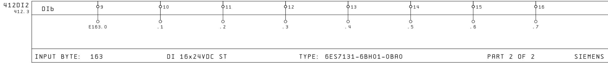
INPUT BYTE: 163                      DI 16x24VDC ST                      TYPE: 6ES7131-6BH01-0BA0                      PART 2 OF 2                      SIEMENS
