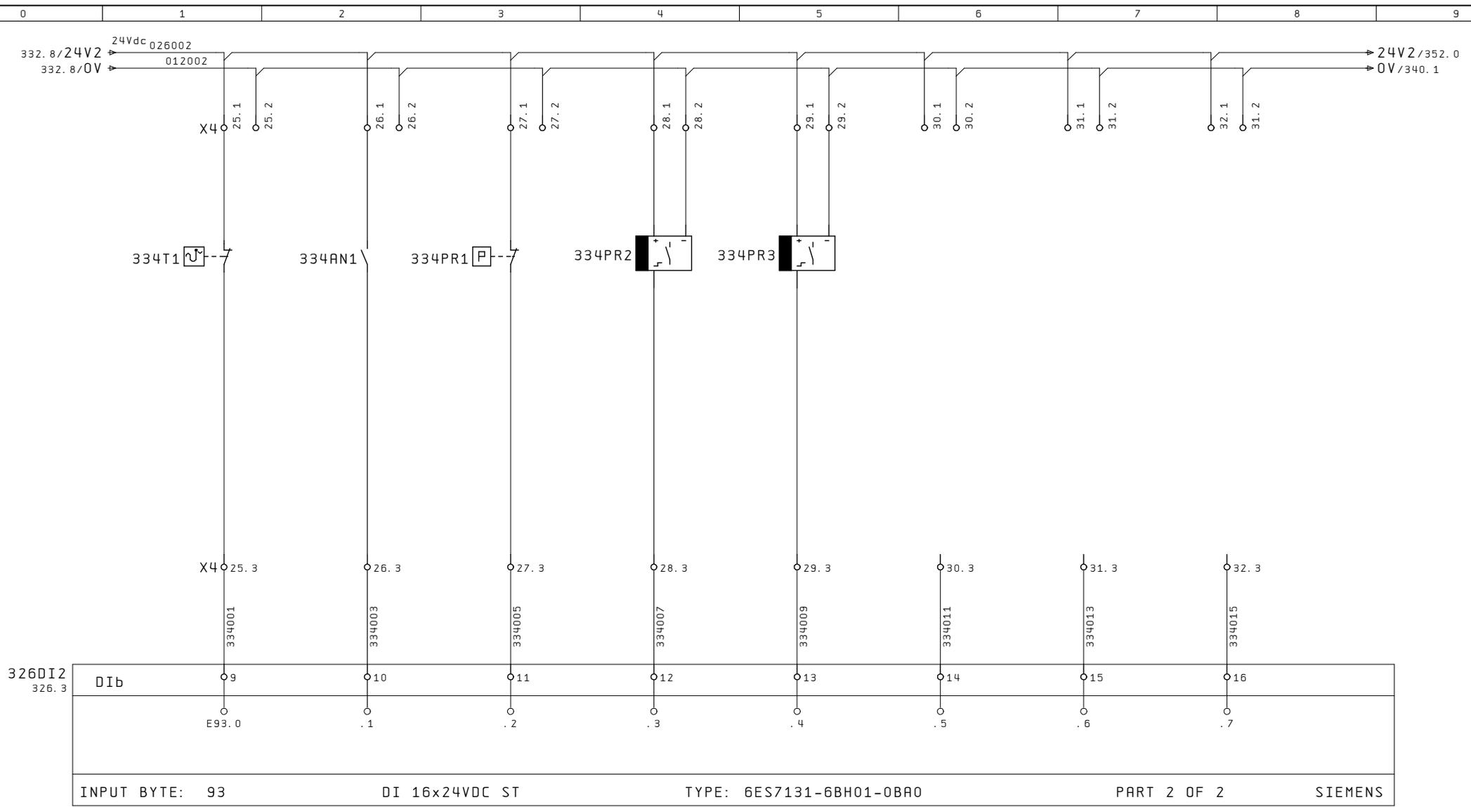
INPUT BYTE: 93      DI 16x24VDC ST      TYPE: 6ES7131-6BH01-0BA0      PART 2 OF 2      SIEMENS
