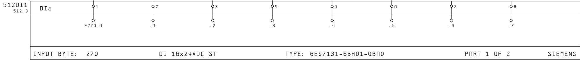
INPUT BYTE: 270      DI 16x24VDC ST      TYPE: 6ES7131-6BH01-0BA0      PART 1 OF 2      SIEMENS
