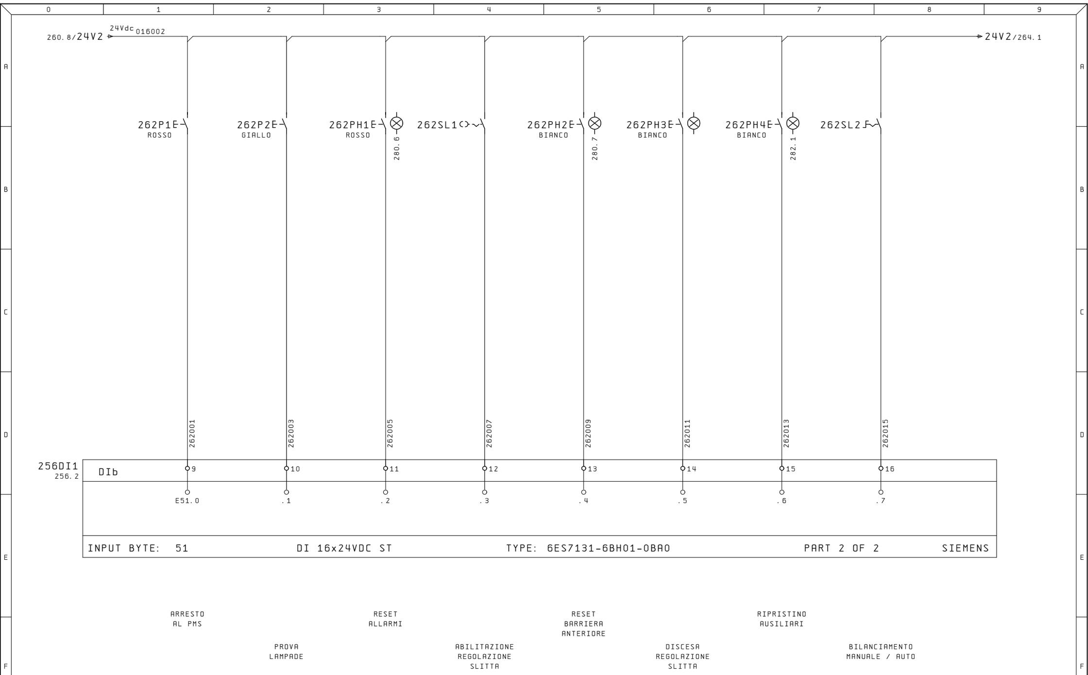
INPUT BYTE: 51      DI 16x24VDC ST      TYPE: 6ES7131-6BH01-0BA0      PART 2 OF 2      SIEMENS
