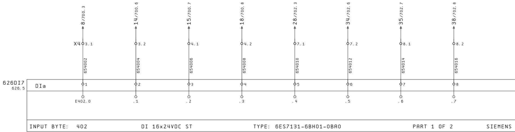
INPUT BYTE: 402      DI 16x24VDC ST      TYPE: 6ES7131-6BH01-0BA0      PART 1 OF 2      SIEMENS
