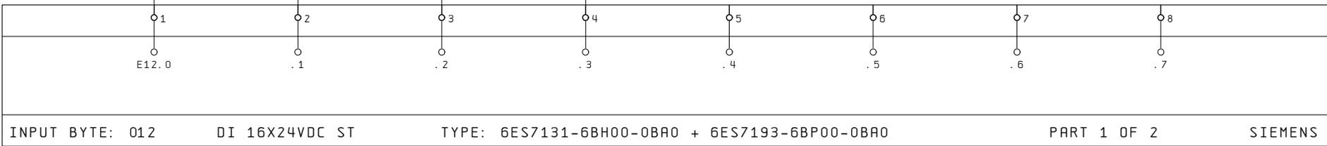
INPUT BYTE: 012      DI 16X24VDC ST      TYPE: 6ES7131-6BH00-0BA0 + 6ES7193-6BP00-0BA0      PART 1 OF 2      SIEMENS
