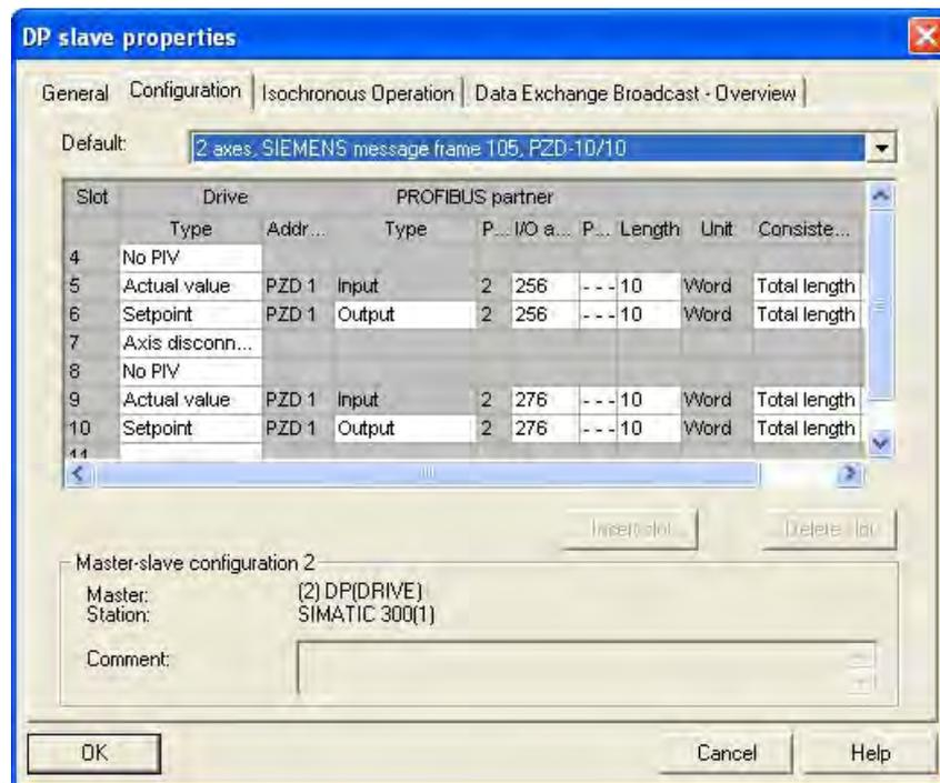
Figure 4-10 Set message frame 105 on the slave
