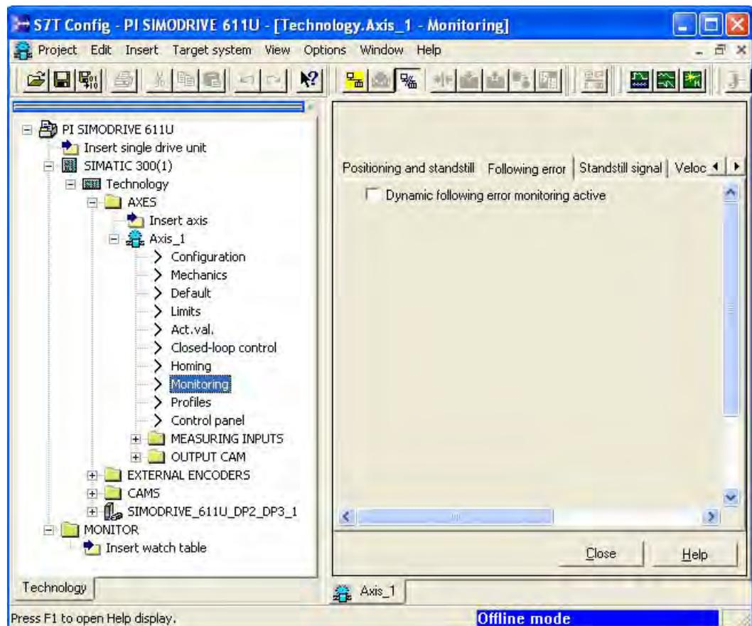
Figure 4-25 Deactivate following error monitoring
