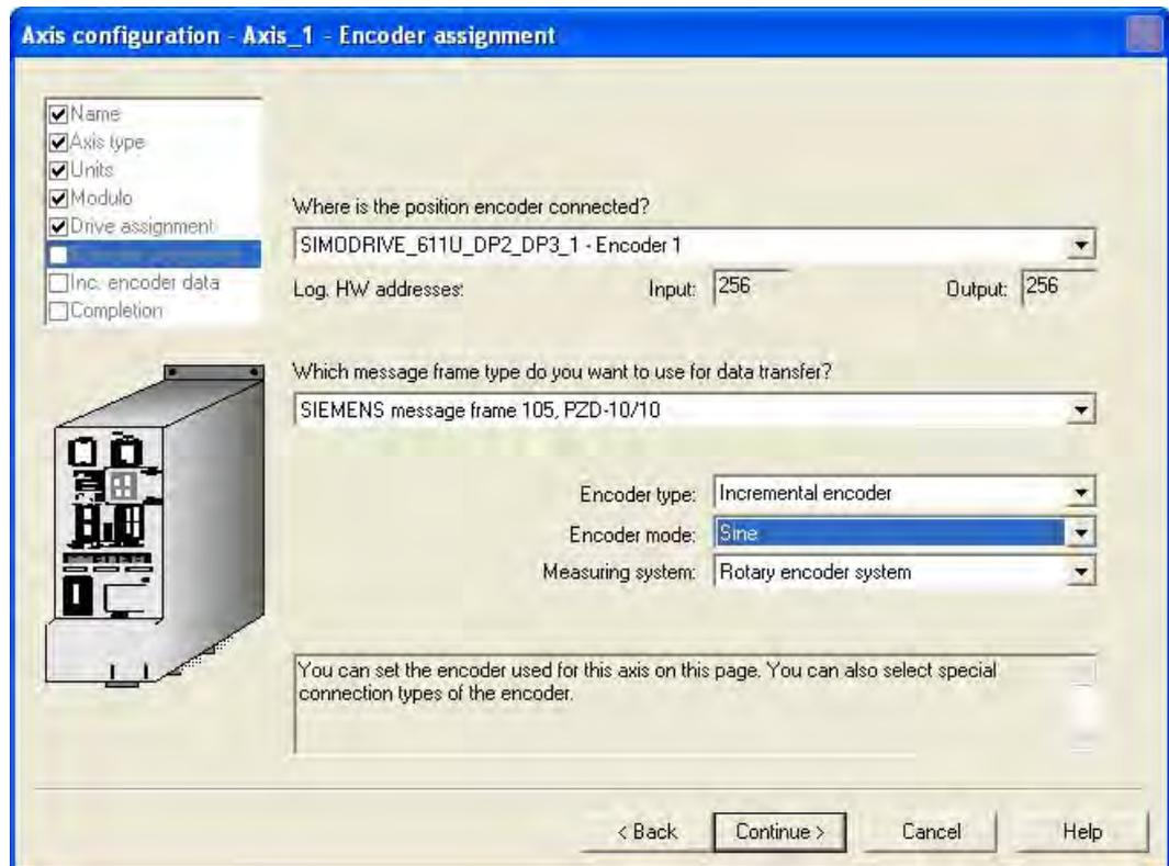
Figure 4-22 Axis configuration in S7T Config (selects the encoder type for incremental encoders)
