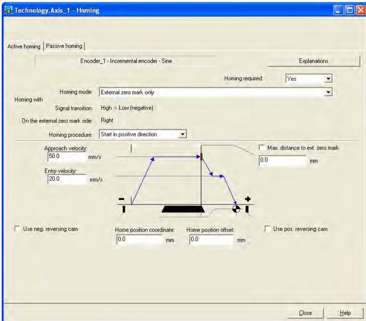
Figure 4-29 Axis homing in STEP 7 (homing mode only external zero mark)
