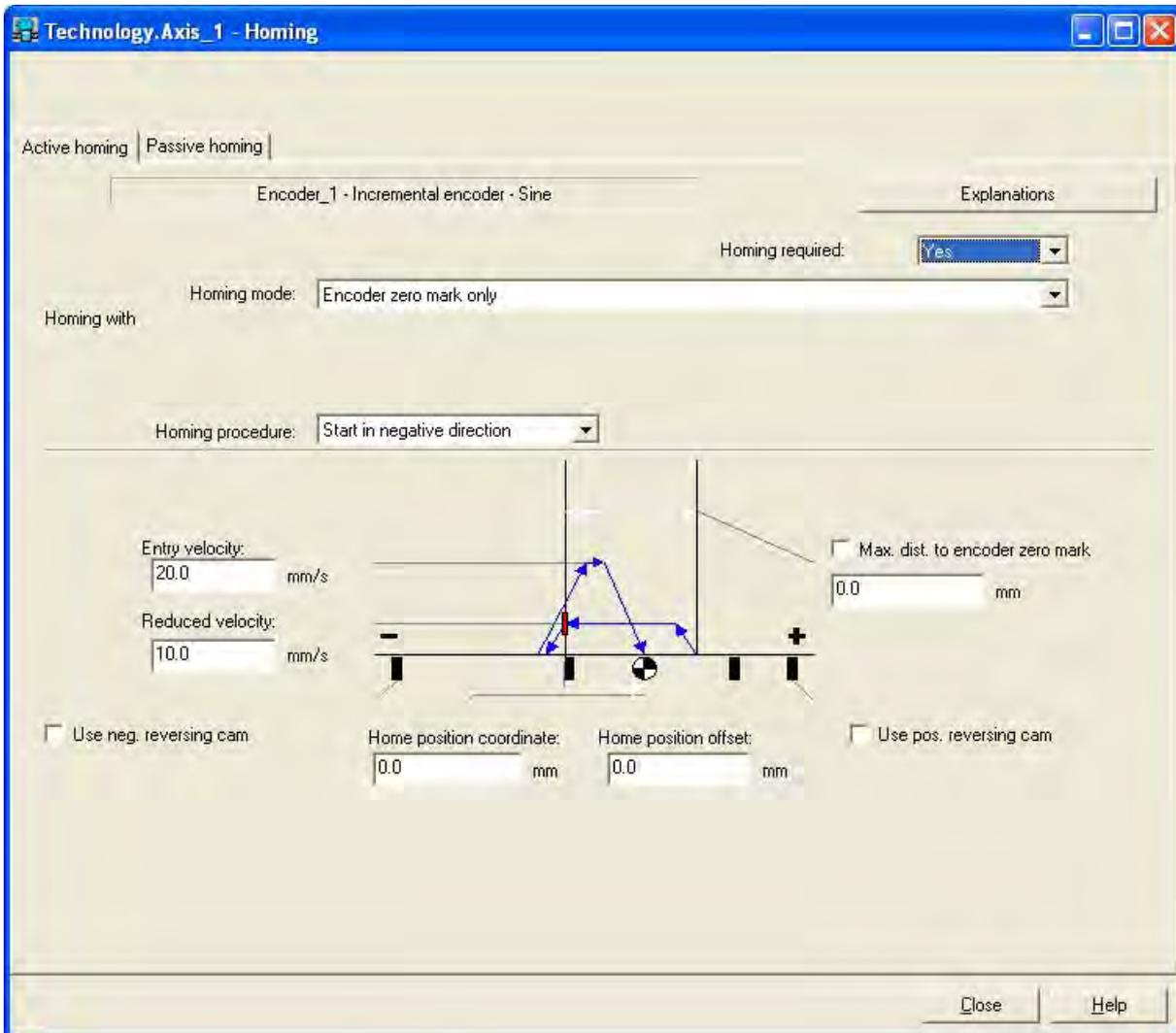
Figure 4-30 Axis homing in STEP 7 (homing mode only encoder zero mark)
