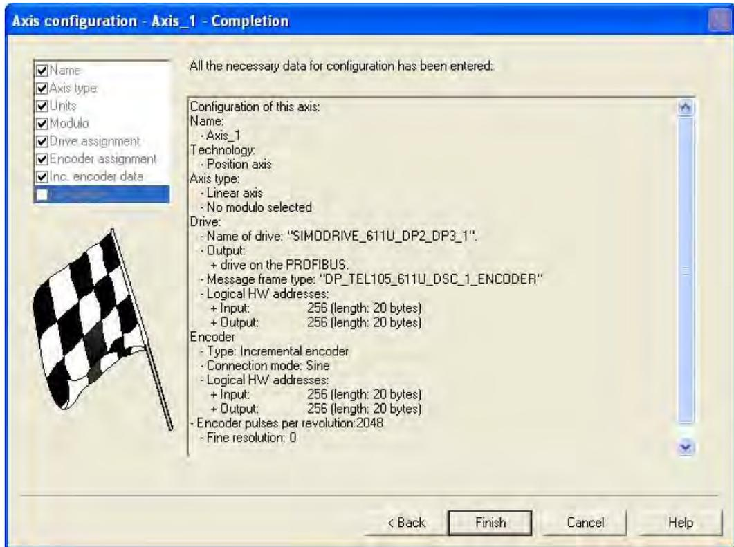
Figure 4-24 Last window of the axis configuration
