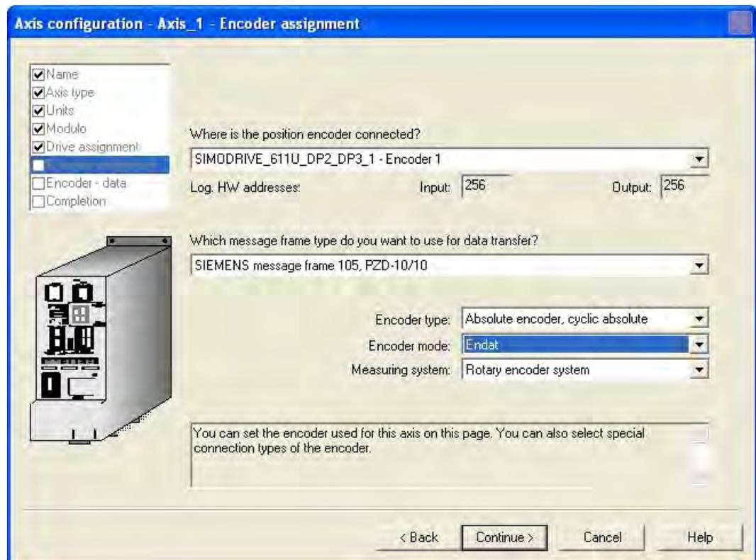
Figure 4-20 Axis configuration in S7T Config (selects the encoder type for absolute encoders)
