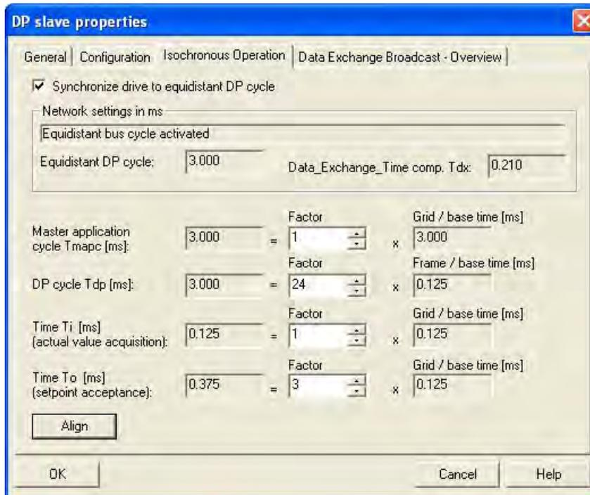
Figure 4-11 Activate clock-synchronized operation
