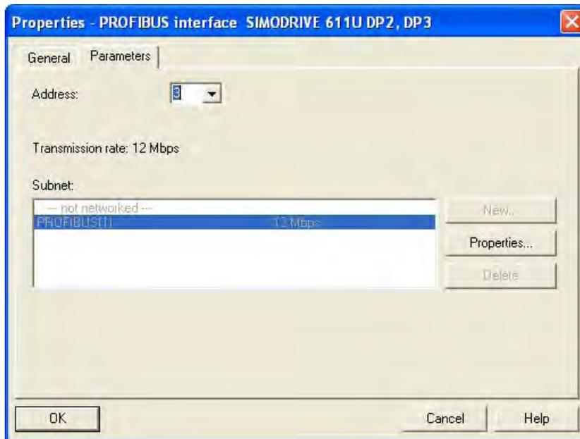
Figure 4-9 Adding a SIMODRIVE 611 universal to the PROFIBUS
