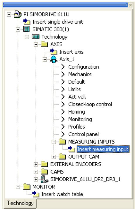
Figure 4-35 Inserting a measuring input
