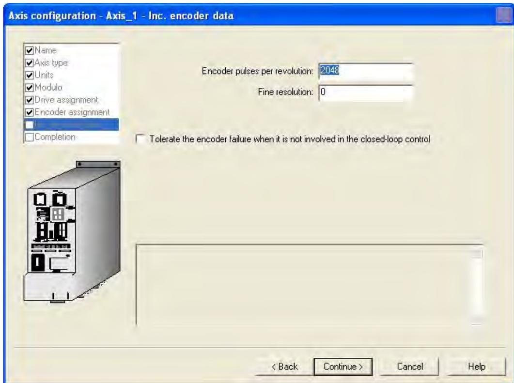
Figure 4-23 Axis configuration in S7T Config (enters the resolution of incremental encoders)
