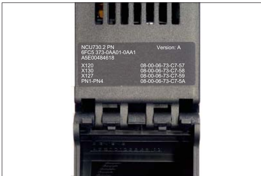
Figure 6-6 MAC addresses of the PROFINET/Ethernet interfaces
