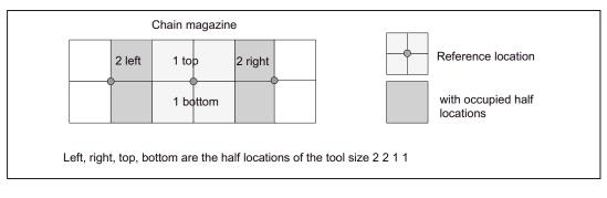
Figure 6-8 Oversized location type for chain magazines
