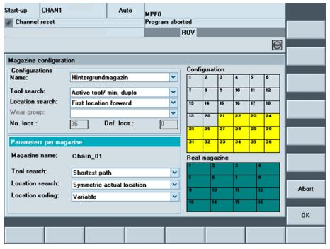
Figure 6-12 Set parameters for each magazine
