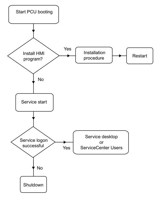
Figure 1-7 PCU bootup diagram (without HMI program)
