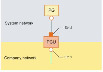
Figure 4-7 Connecting a PG directly to a PCU
