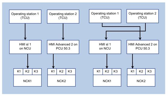
Figure 2-4 Switchover (solution line)
