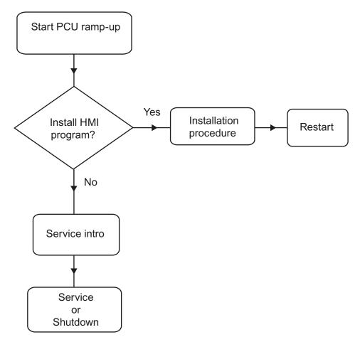
Figure 1-6 PCU bootup diagram (without HMI program)
