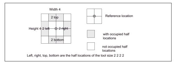
Figure 6-10 Oversized location type with free half locations for box magazine
