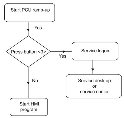
Figure 1-7 PCU bootup diagram (HMI program installed)
