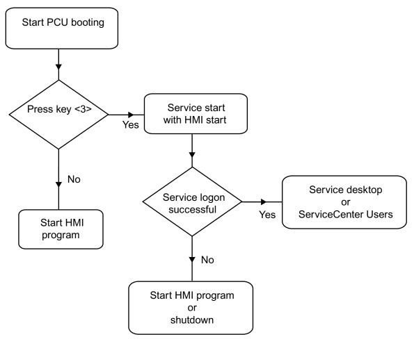
Figure 1-8 PCU bootup diagram (HMI program installed)
