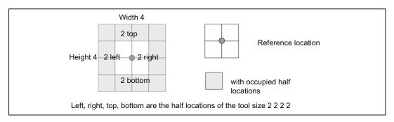
Figure 6-9 Oversized location type for box magazines
