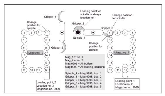
Both magazines can be loaded via Spindle\_1. Loading point\_1 is only assigned to Magazine\_1 and Loading point\_2 is only assigned to Magazine\_2.
