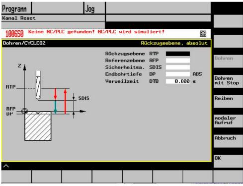
Figure 2-8 Appearance in HMI Advanced
