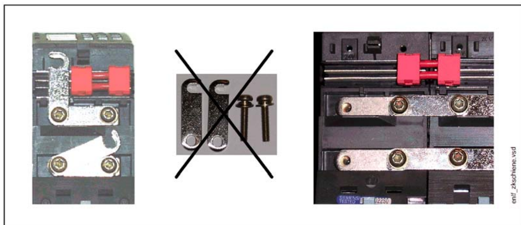
Figure 2-1 Removal of the DC link bridge
