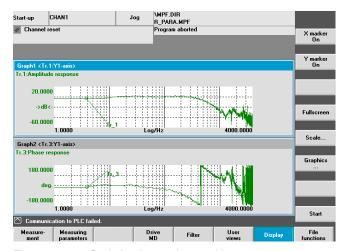
Figure 11-5 Optimized speed control loop
