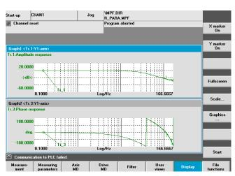
Figure 11-6 Optimized position control loop
