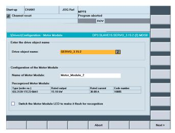
Figure 8-42 Menu "Drives > Configuration" "Motor with externally supplied motor) (Next 1)
