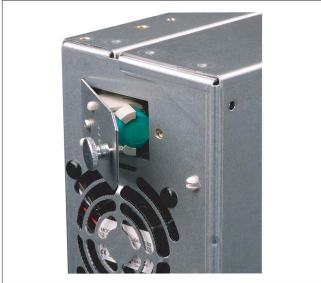
Figure 13-34 (A) Opening the battery compartment
