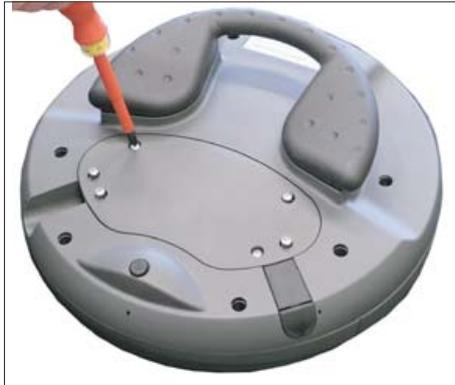
1. Open the cable duct cover by unscrewing the six PT screws (4 x 20 mm) approximately 1 cm. To do this, use a crosstip size 2 screw driver.
