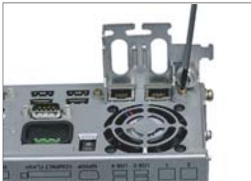
2. Secure the ETH strain relief on the PCU by tightening the two screws with a Torx screwdriver T10.
