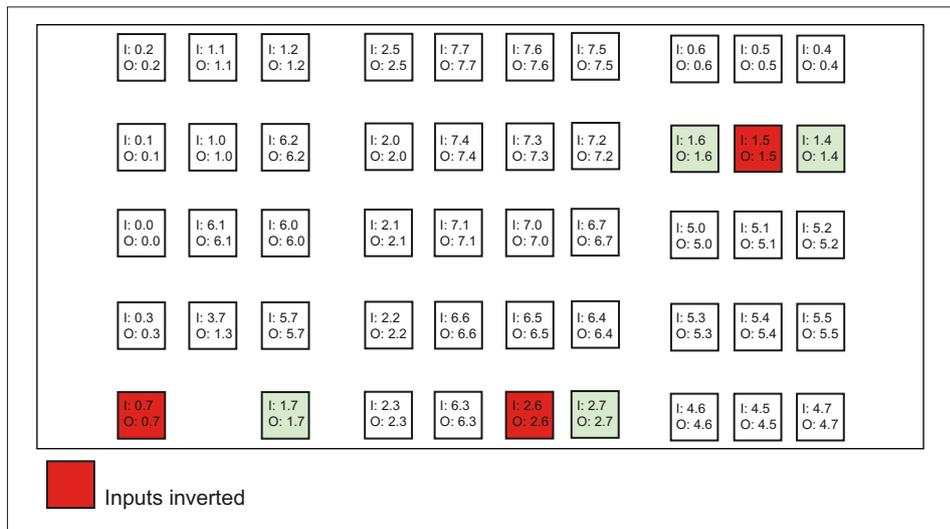
Figure 2-7 Inputs and outputs of the MCP 310 PN keyboard
