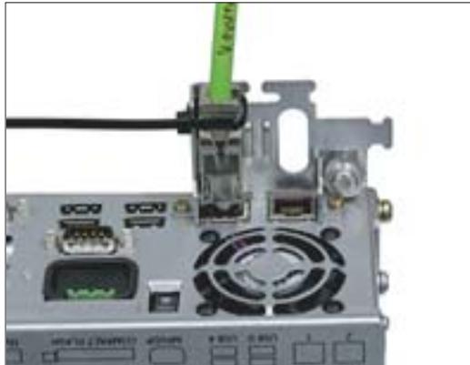
4. Secure the Ethernet cable at the ETH strain relief with a cable tie.
