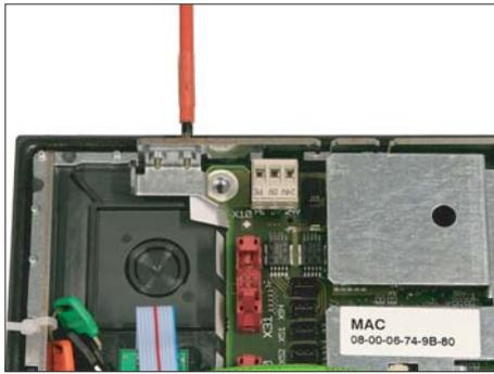
2. Remove the two fastening screws (M3) using a TX 10 screwdriver.
