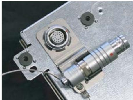
3. Tighten the retaining nut and insert the terminating connector into the bracket.
