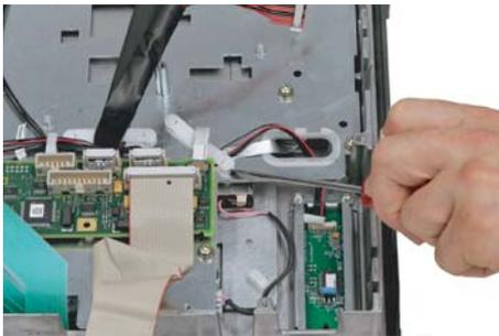
6. Remove the retainer for the cable running between the keyboard controller and mouse.
