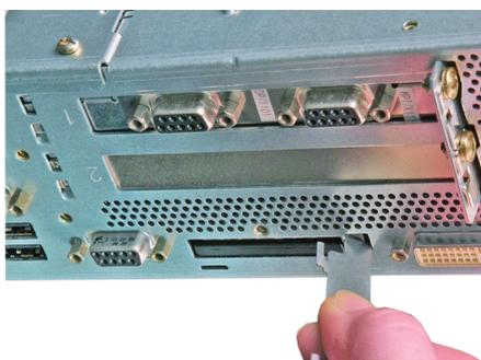
3. Remove the CompactFlash card.
