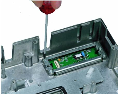
10. Loosen the 4 screws (M3) on the holder for the mouse board. Lift off both the holder and the mouse board.
