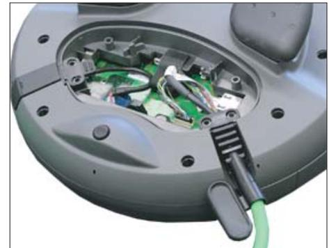
5. Put the cable duct cover on and secure it by tightening the six screws.
