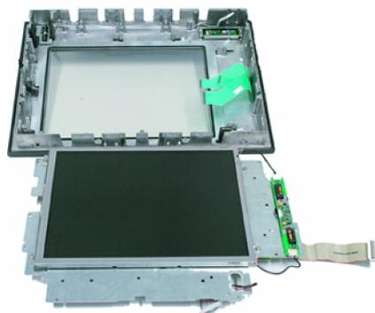
14. Lay the display support down on its back to avoid damaging the display.
