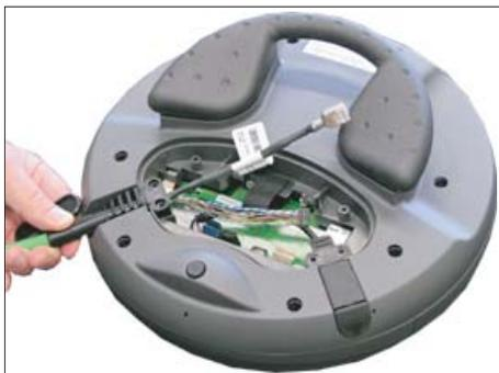
2. Insert the connecting cable into the cable inlet that suits your intended application (left or right).
