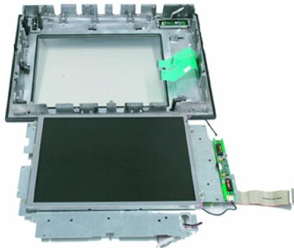
13. Lay the display support down on its back to avoid damaging the display.
