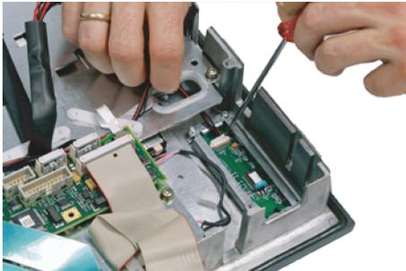
4. Undo the connection between the keyboard controller and the mouse by carefully pushing the connector back with a screwdriver.
