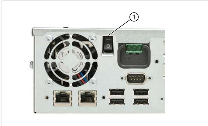
Figure 13-3 PCU 50.3 On/Off switch
