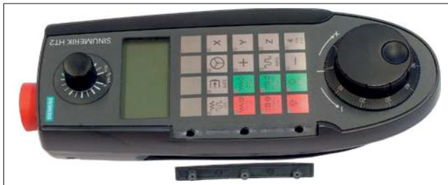
1. Release the three cross-recessed screws (PT2, 5x14). To do this, use a crosstip size 1 screw driver (PH1). Each of the screws has a marking.
