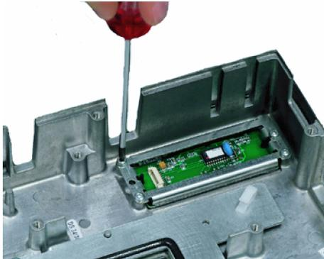
10. Loosen the 4 screws (M3) at the support for the mouse board using a Torx screwdriver T10. Lift off both the holder and the mouse board.
