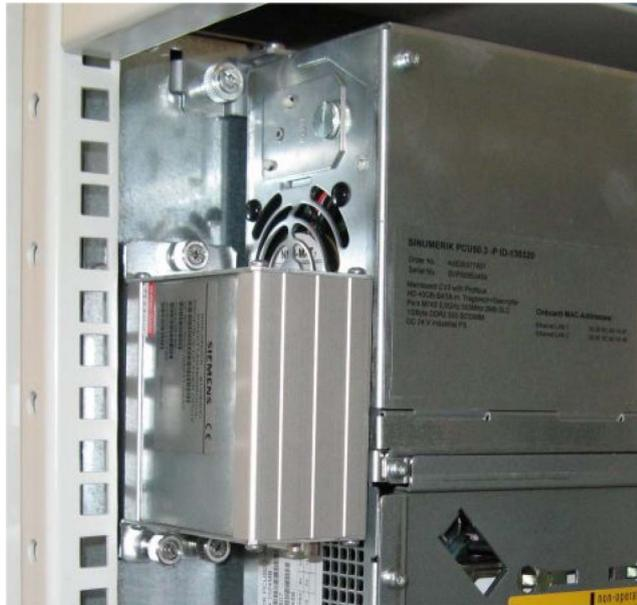
Figure 12-15 Direct key module after installation
