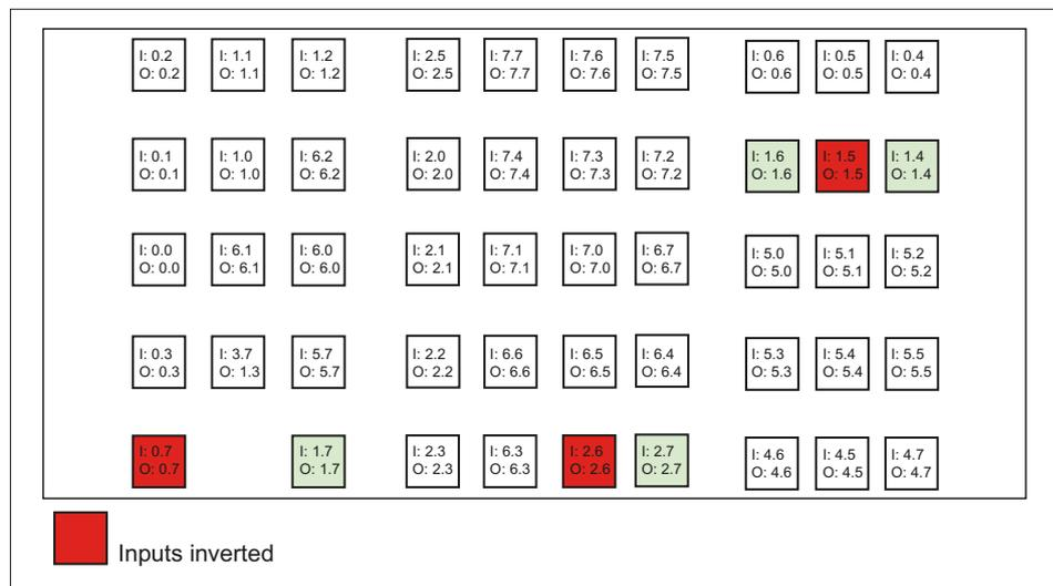
Figure 3-7 Inputs and outputs of the MCP 310 keyboard
