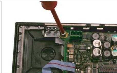
1. Remove the fastening screw (M5) using a TX 25 screwdriver.
