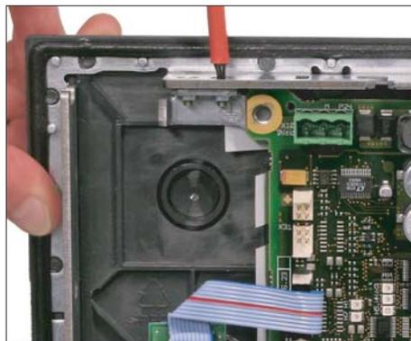
2. Remove the two fastening screws (M3) using a TX 10 screwdriver.
