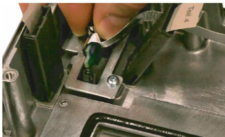
14. Remove the USB interface by sliding up both retaining clamps and pulling out the board.
