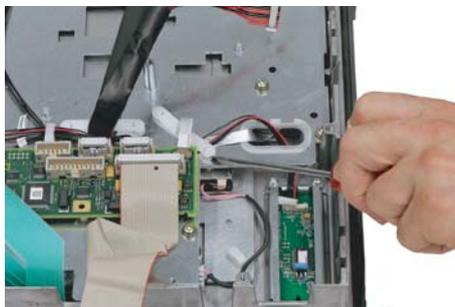
9. Remove the retainer for the cable running between the keyboard controller and mouse.
