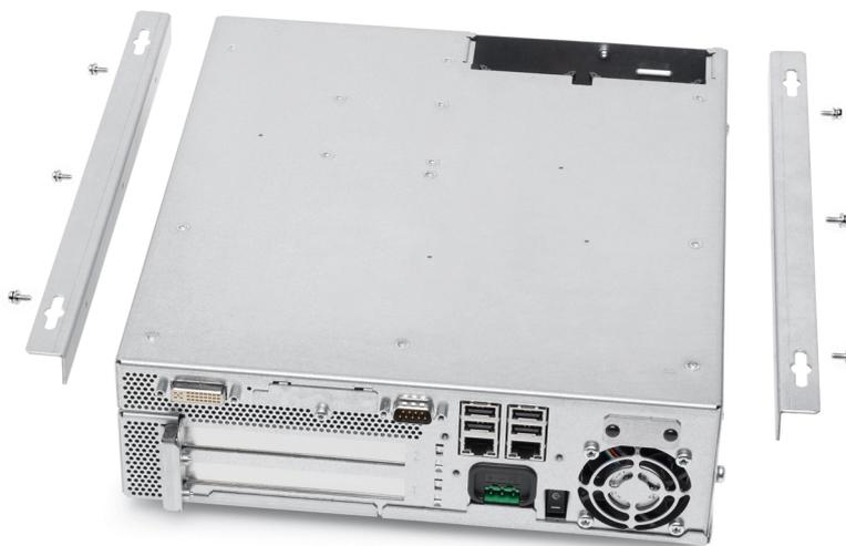
Figure 14-13 PCU 50.5 with bracket for flat mounting
