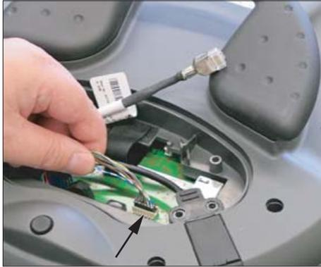
3. Press the plug connector firmly into the power supply socket (1).
