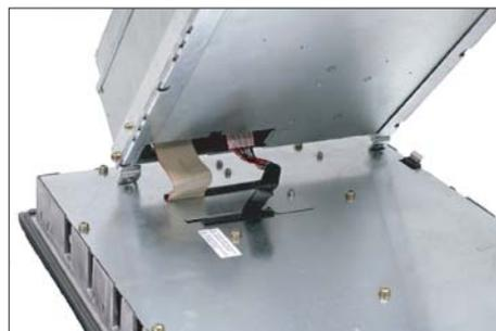
6. Swing the PCU in the direction of the OP 015A, making sure that the cables are folded correctly.
