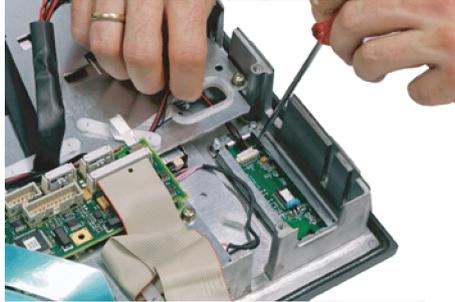
8. Undo the connection between the keyboard controller and the mouse by carefully pushing the connector back with a screwdriver.
